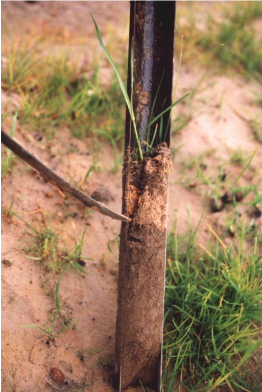
Fig. Visible plant root systems growing through the biogenic layer and entering the top layers of flotation sludge under the stabilizing layer.
