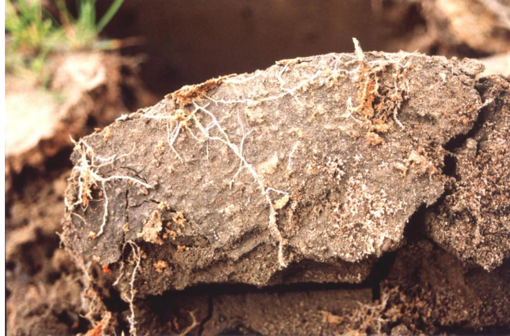
Fig. Visible plant root systems growing through the biogenic layer and entering the top layers of flotation sludge under the stabilizing layer.
