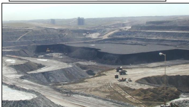
North Antelope Rochelle Mine 60 m overburden 20 m coal 3:1 ratio
