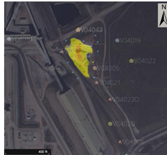
3D Conceptual Site Model of PFAS in Soil and Groundwater Fire Training Area (FTA) Plan View
