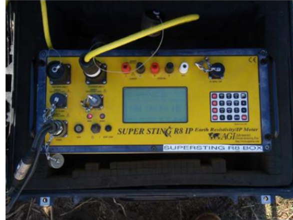
Figure 3. AGI Supersting RES/IP Meter
