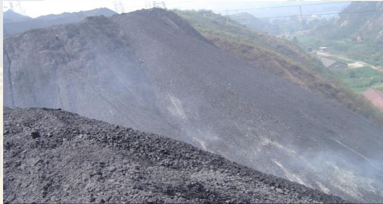
Spontaneous combustion and explosion of coal gangue heaps
