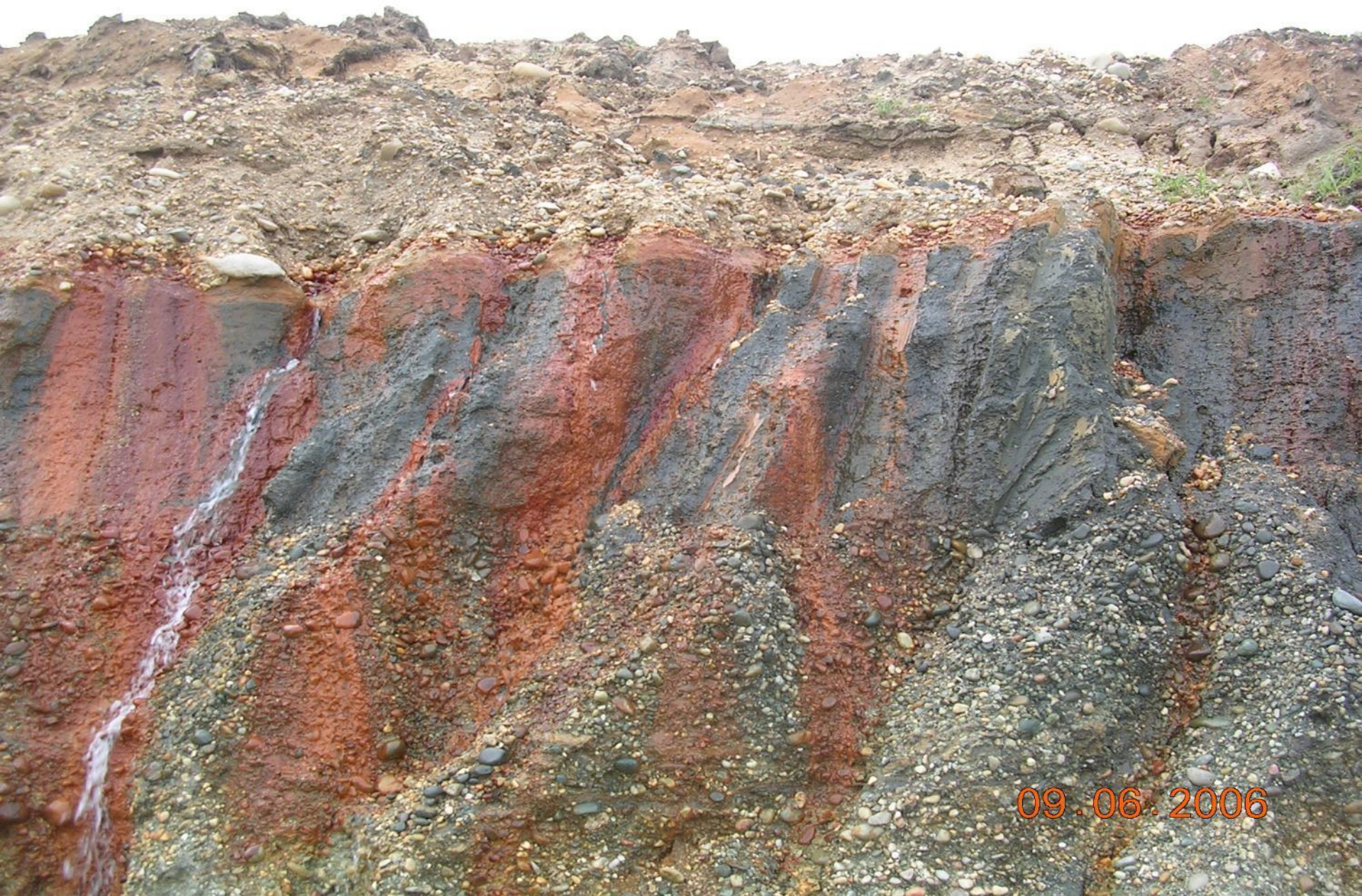
Typical abrupt contact between Plio/Pleistocene gravels and underlying Miocene ASS materials (Eastover fm). Fe-stone (ferricrete) often found at contact.
