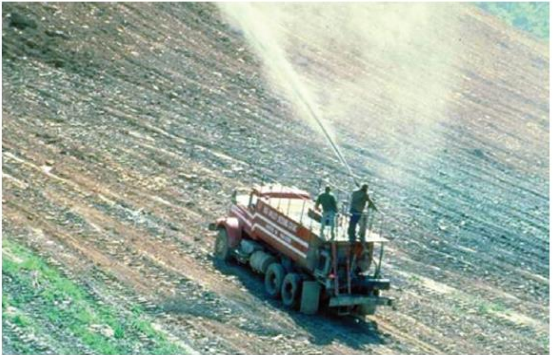
Figure 5. A hydroseeder applying seed in a fertilizer slurry while revegetating a surface coal mine.
