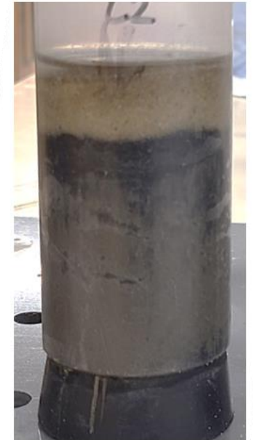
Core from Thin-layer AC Cap (5 wt%) & 2 cm Sand Cap
