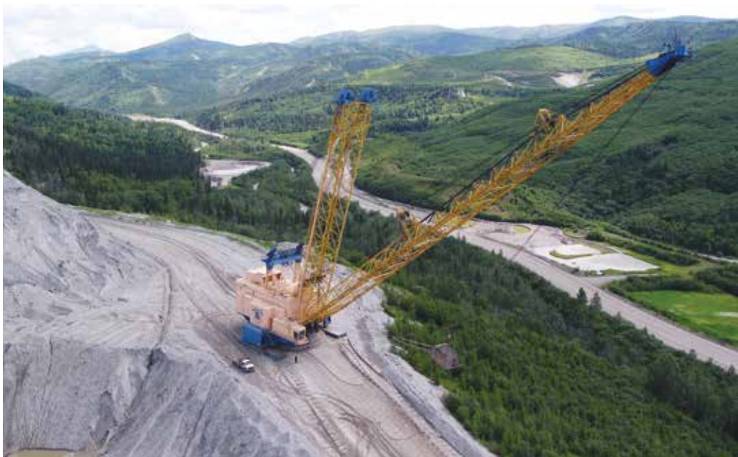
Figure 2. Bucyrus-Erie 1300W dragline, named “Ace in the Hole,” moves the overburden overlying the coal seams at Poker Flats and Two Bull Ridge Mines.
