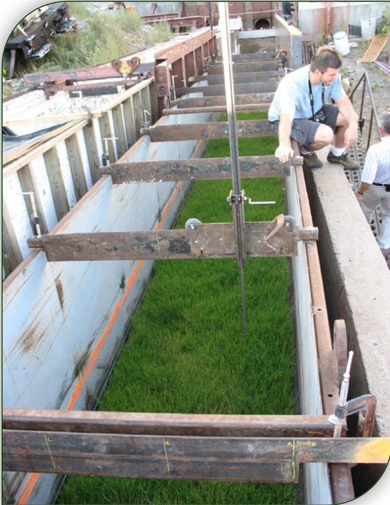
Flume test box in place
