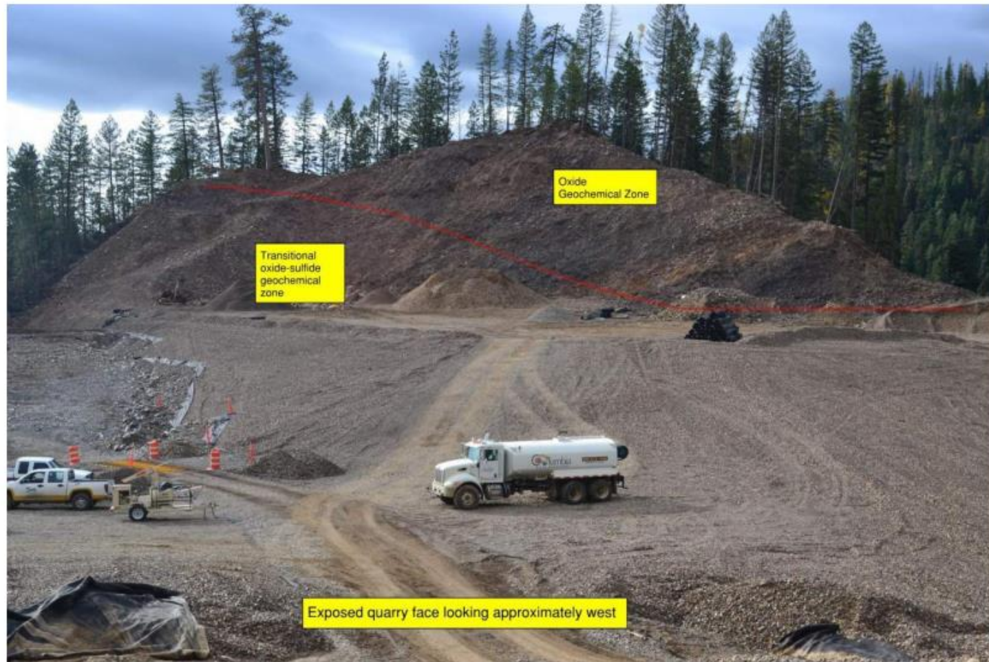
Figure 2. View of EFNW WCA quarry showing approximate location of oxide and transitional oxide-sulfide geochemical zones
