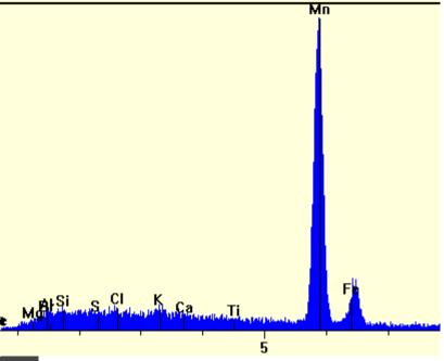
Manganese concentrations exiting the final adsorption vessels were much less than influent concentrations, indicating manganese precipitation within the media beds
