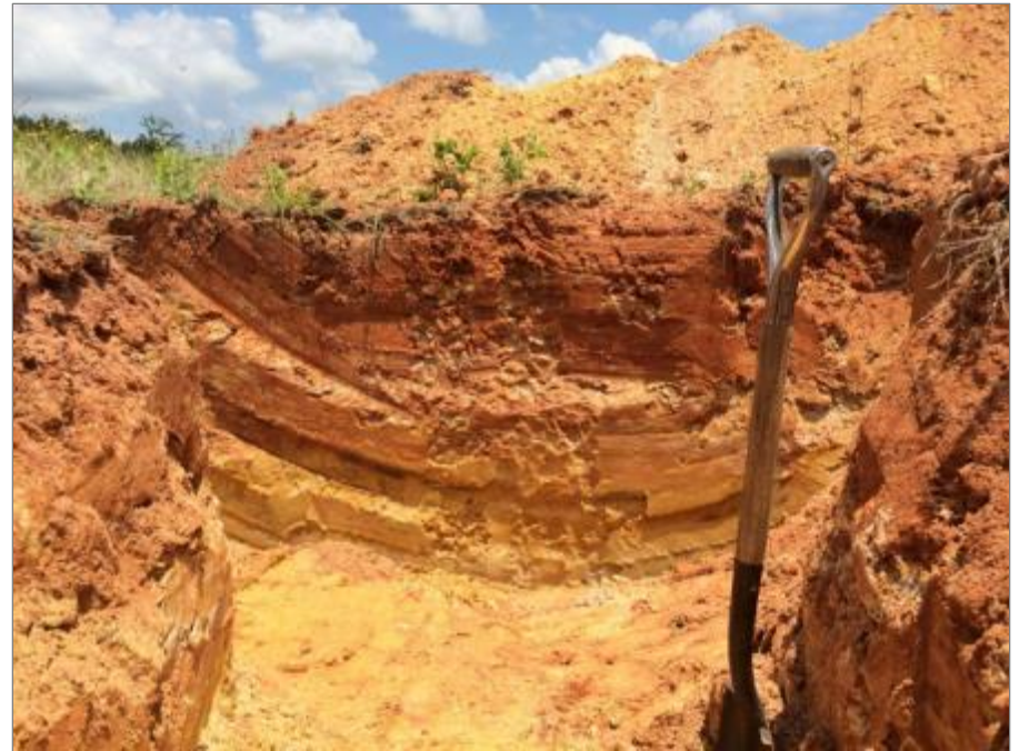
Example of Soil Test Pit
