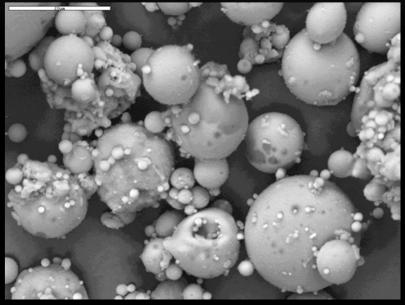
• Bottom ash "rougher" particles and higher amounts of carbon
