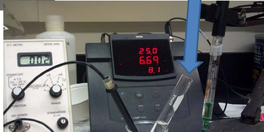
Each Sample is Analyzed for Saturated Paste Electrical Conductance (EC) and pH
