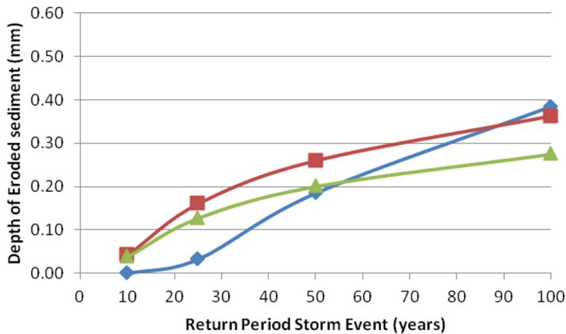
**WEPP Erosion Predictions - Hillslopes with 10 slope points defined**
