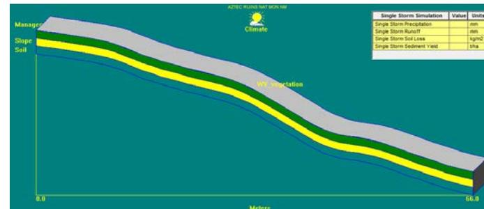
Hillslope defined by simplified S-shape using average slope
