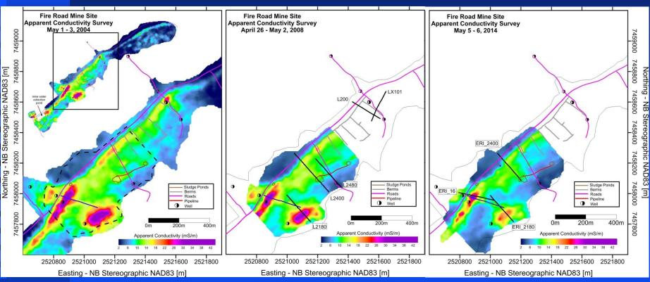
Electrical conductivity of the waste rock backfill appears to be decreasing over time
