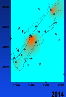
**Geophysical Investigations** UNB Earth Sciences Field Camp since 2000 Electrical resistivity imaging (ERI) and electromagnetic apparent conductivity: ◆ map lateral and vertical variations in AMD and sludge concentration within the mine site Conductivity is proportional to ion concentration, ion valence, and ion mobility. AMD, sludge and clays have high electrical conductivity compared to natural ground waters
