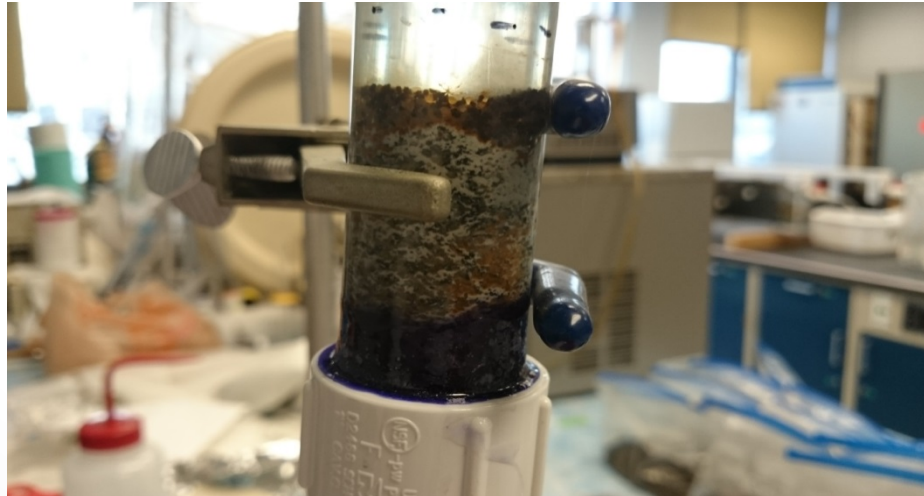
Rust trapped inside the WTR-filter bed during treatment
