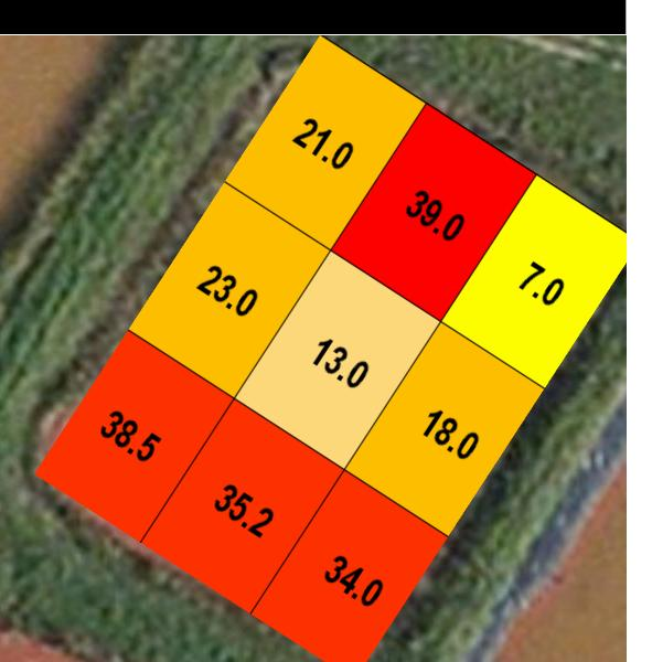
Solids gradient observed along design flow path for surface flow wetland.
