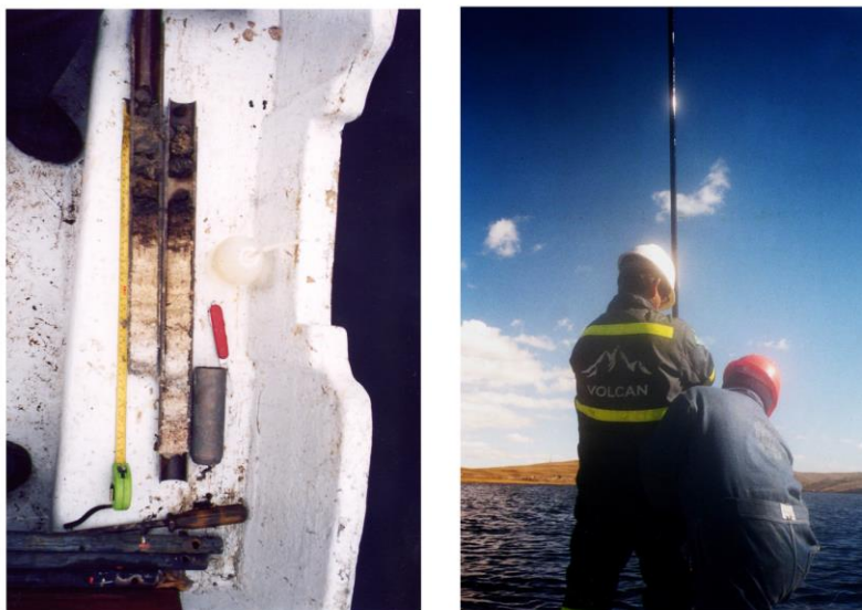
Figure 2: A) The unscrewed and opened corer with soil sample CPY007 from Lake Huaygacocha. B) Hoisting the corer with two persons.
