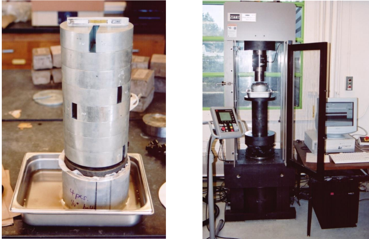
Figure 2. Specimen compaction using free weights and in a hydraulic press.
