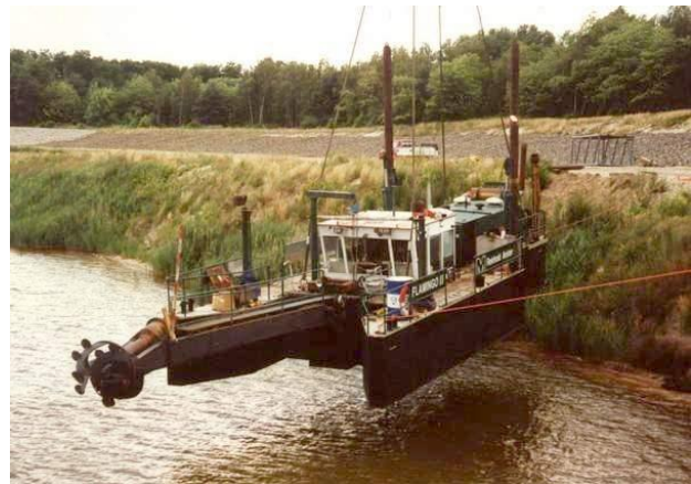
Figure 4. Excavator used in the re-suspension tests (courtesy of eta AG engineering Cottbus).
