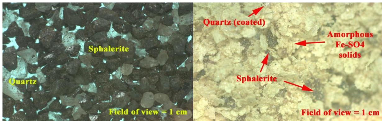
Figure 6. a)Unreacted coarse-grained VMS-WL-01 sphalerite (dark grains; grain diameters approximately 1 mm), and b)VMS-WL-01 after 8 months of reaction. Yellow material consists primarily of iron- and sulfate-rich amorphous phases.
