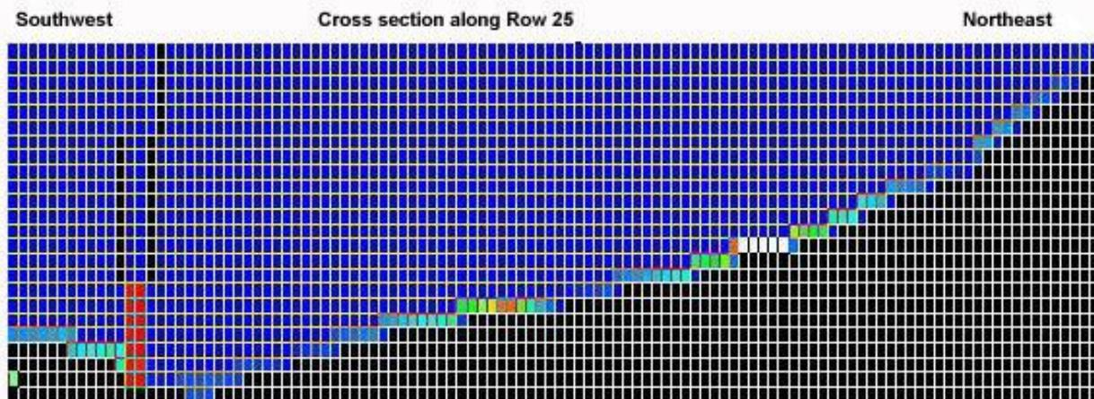
Figure 3. Color flood image of velocity along the longitudinal profile of the Irwin Basin Groundwater Vistas model. Velocities (ft/day): White >20; Red 18-20; Orange 16-18; Yellow 14-16; Lime-green 9-14; Aqua 4-7; Dark Blue 0-3.
