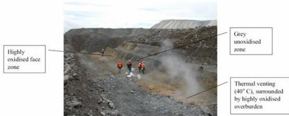
Figure 3: Exposure showing oxidized face zone and convective venting from a sloping coarse layer which appeared to have accelerated oxygen transfer within the stockpile.
