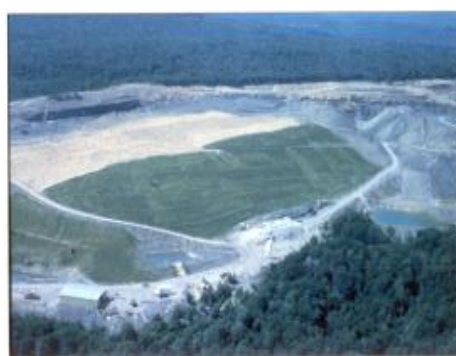
Figure 1d. Adjacent site to 1c during re-mining showing surface regrading and revegetation in foreground. Active coal removal area is in background.
