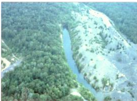
Figure 1c. Abandoned mine lands in central Pennsylvania showing unvegetated acid-forming spoil and impounded pit water.
