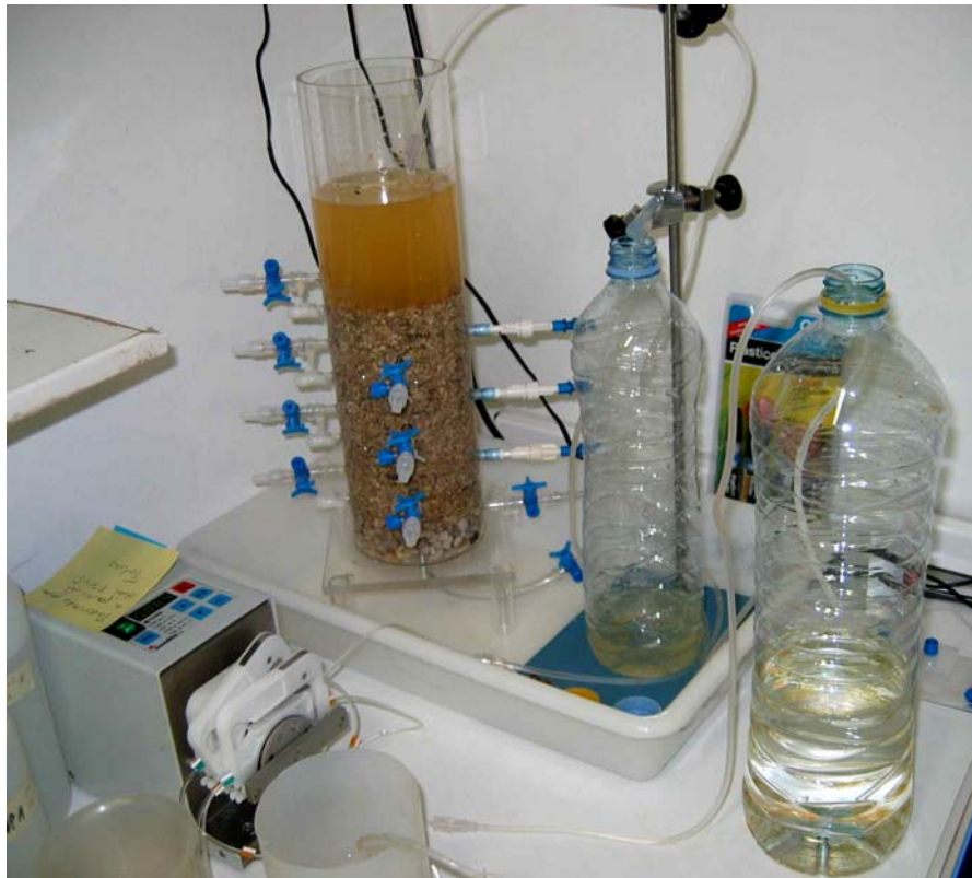
Figure 1. A) Design of laboratory columns, B) Column #1 at the start of the experiment with input container (right), output container with overflow pipe (middle) and peristaltic pump (left).
