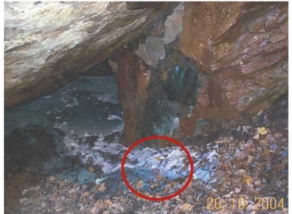
Figure 7. White (04PKHL5-A) and blue (-B & -C) amorphous or weakly crystalline glaucocerinite precipitates along decline to perched adit pool in Union mine workings.
