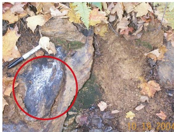
Figure 3. Melanterite salts (04Smith1-1) on weathered ore of the uppermost waste dump (04Smith1) at the Smith Mine.
