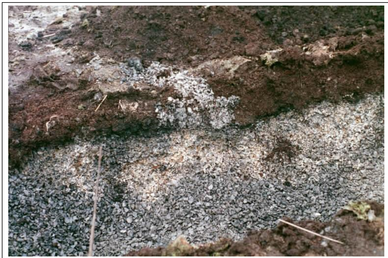
Figure 4. Well developed white coating on upper part of limestone bed, and black layer at base of compost. Area at left is obscured by loose limestone. Spilled compost covers limestone in a spot near right, and spilled limestone covers compost in center.
