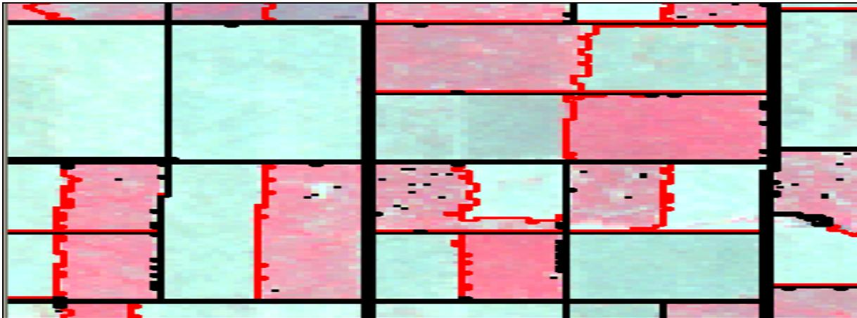
Figure 2. Object segmentation results for the field strip level (red vector lines). Black parameter lines represent taxable field boundaries.
