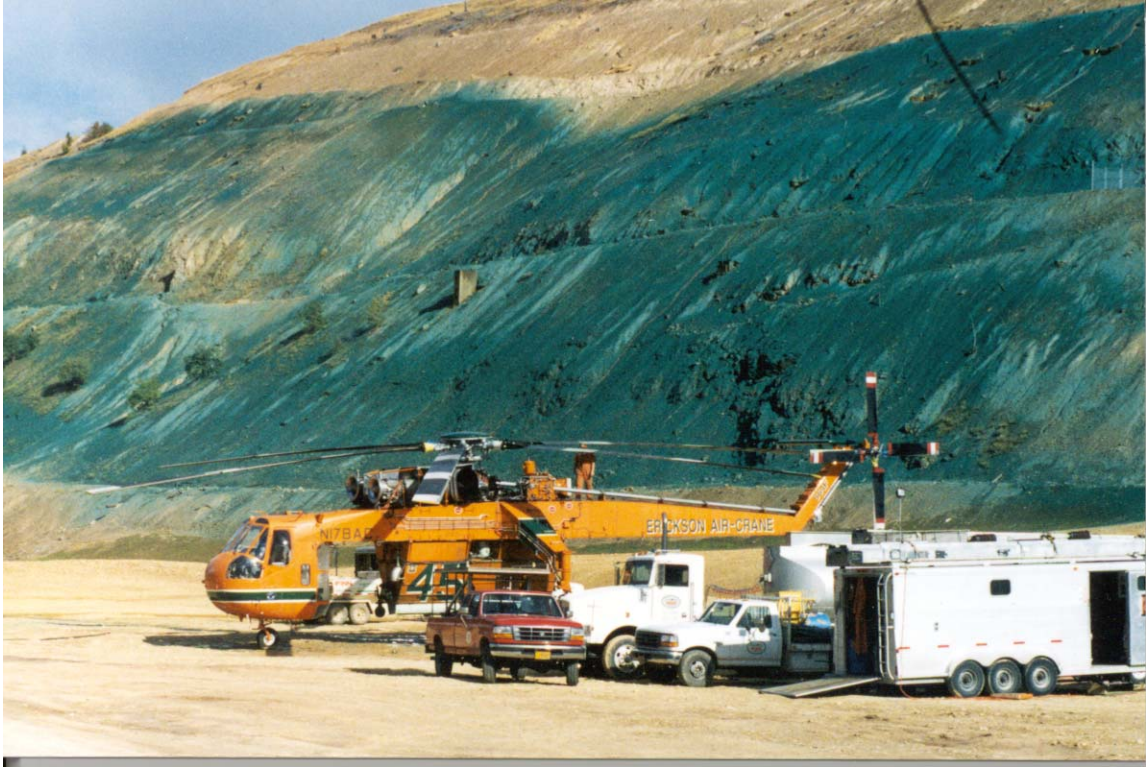
Figure 2. Steep slopes and poor access resulted in the use of aerial application techniques on the hillsides. Sikorski helicopters were used to apply most of the hillsides prescriptions. Although per hour costs are high, application rates were much higher than with other air frames and per hectare application costs were effective. Note hydroseed materials on background slopes.
