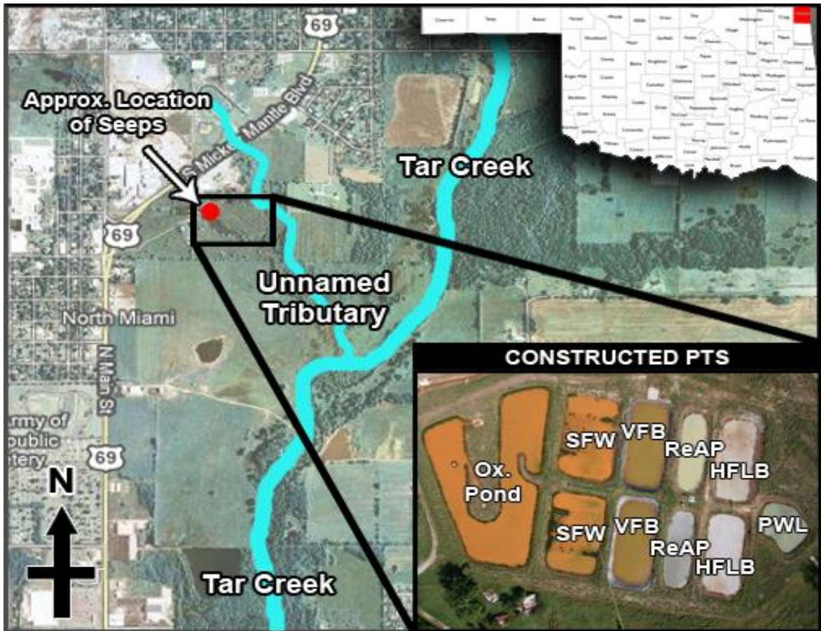
Figure 1. Location map for mine drainage site. Mine water flows from seeps to Unnamed Tributary and to Tar Creek. Currently, PTS intercepts mine drainage from seeps before it reaches Unnamed Tributary. Key- Oxidation Pond: Ox. Pond, Surface Flow Wetland: SFW, Vertical Flow Bioreactor: VFB, Re-aeration Pond: ReAP, Horizontal Flow Limestone Bed: HFLB, Polishing Wetland: PWL.
