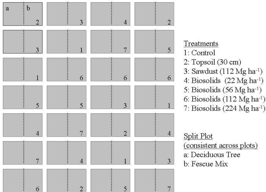
Figure 1. Treatments in the controlled overburden placement experiment at the Red River Coal Mine, Wise County, Virginia.
