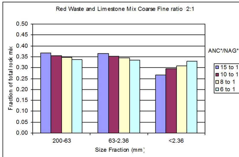
Figure 3. Relative amounts of rock within each particle size fraction for the Red waste and Limestone mixes at a Coarse to Fine ratio of 2:1 for different bulk ANC\*/NAG\* ratios expressed as a fraction of the total rock mass in the mix.
