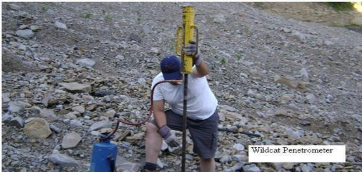
Figure 14: Wildcat Dynamic Cone Penetrometer field set up
