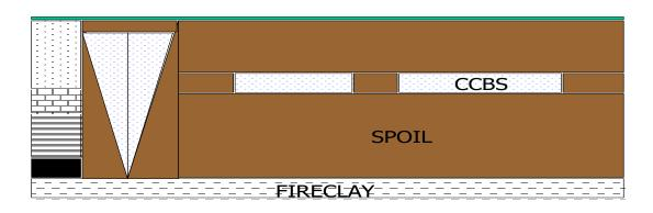
Figure 2. Typical cross-section of CCB placement at a reclaimed coalmine site.
