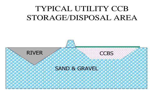
Figure 1. Typical cross-section of an electric utility disposal site where toxic leachate has occurred.
