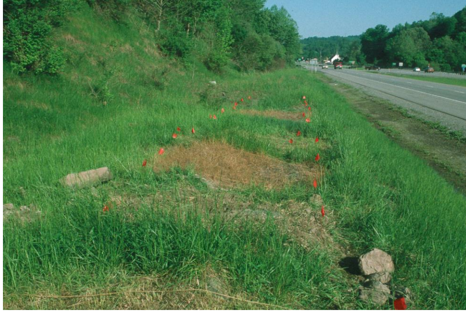
Figure 4. Overview of plots located at Weston, WV. It is located approximately 3m above the road. Due to spatial constraints this site was laid out in a linear arrangement. The different surface treatments applied to the plots can be seen. In the foreground is a tilled plot, then an herbicide treated plot, a mowed plot, and another herbicide treated plot.
