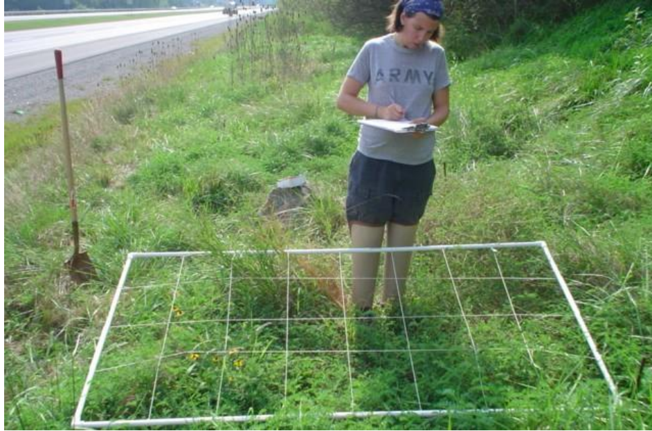
Figure 5. Plots were surveyed using the Daubenmire cover class system to determine total cover and cover by species. For ease, a portable sampling grid was designed with 0.25\text{m}^2 subplots. Four randomly selected subplots were surveyed and results were averaged to determine plot cover.
