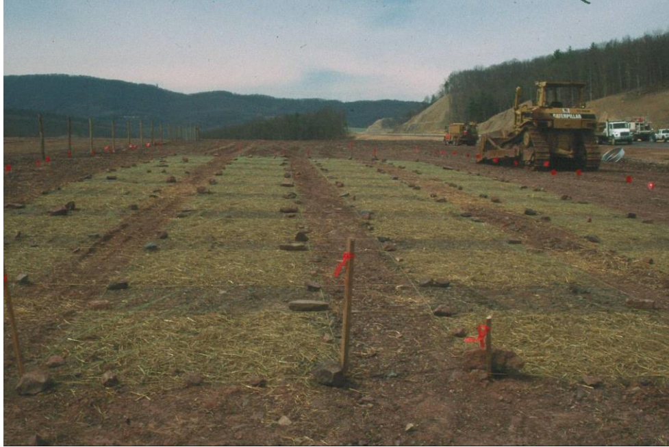
Figure 2. Overview of plots located at Baker, WV. This site was approximately 1 year old prior to plot establishment and had little vegetative cover. The soil was very compact and rocky. Plots were arranged in an 11x29 m rectangle (four rows of ten plots).
