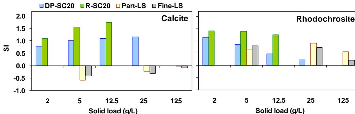
Figure 5. Saturation indices (SI) for calcite ( $\text{CaCO}_3$ ) and rhodochrosite ( $\text{MnCO}_3$ ) in systems containing SMIW with initial Mn of 10 mg/L and pH 3.0, treated with DP-SC20, R-SC20, particulate, and fine limestone.
