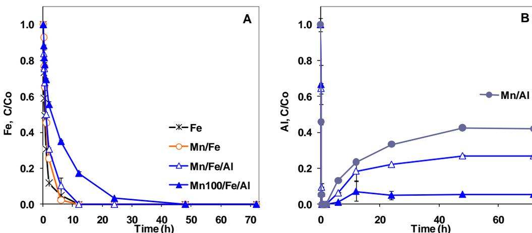
Figure 4. Iron (A) and aluminum (B) changes in reactors containing SMIW and 5 g/L of DP-SC20. Initial metals concentrations were 10 mg/L each, except for Mn100/Fe/Al (panel B), where  $\text{Mn}_o = 100$  mg/L, and initial pH was 3.0. Detailed experimental conditions for each test are provided in Table 2.
