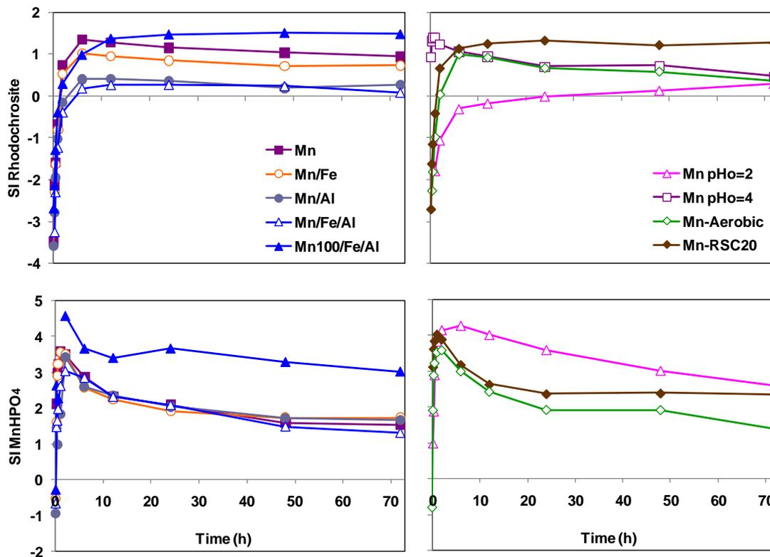
Figure 6. SI values for rhodochrosite ( $\text{MnCO}_3$ ) and  $\text{MnHPO}_4$  in reactors containing SMIW and 5 g/L of DP- or R-SC20. Initial metal concentrations were 10 mg/L each, except for Mn100/Fe/Al (central panel), where  $\text{Mn}_0 = 100$  mg/L. Initial pH was 3.0, unless otherwise specified (right panel). Detailed experimental conditions for each test are provided in Table 2.
