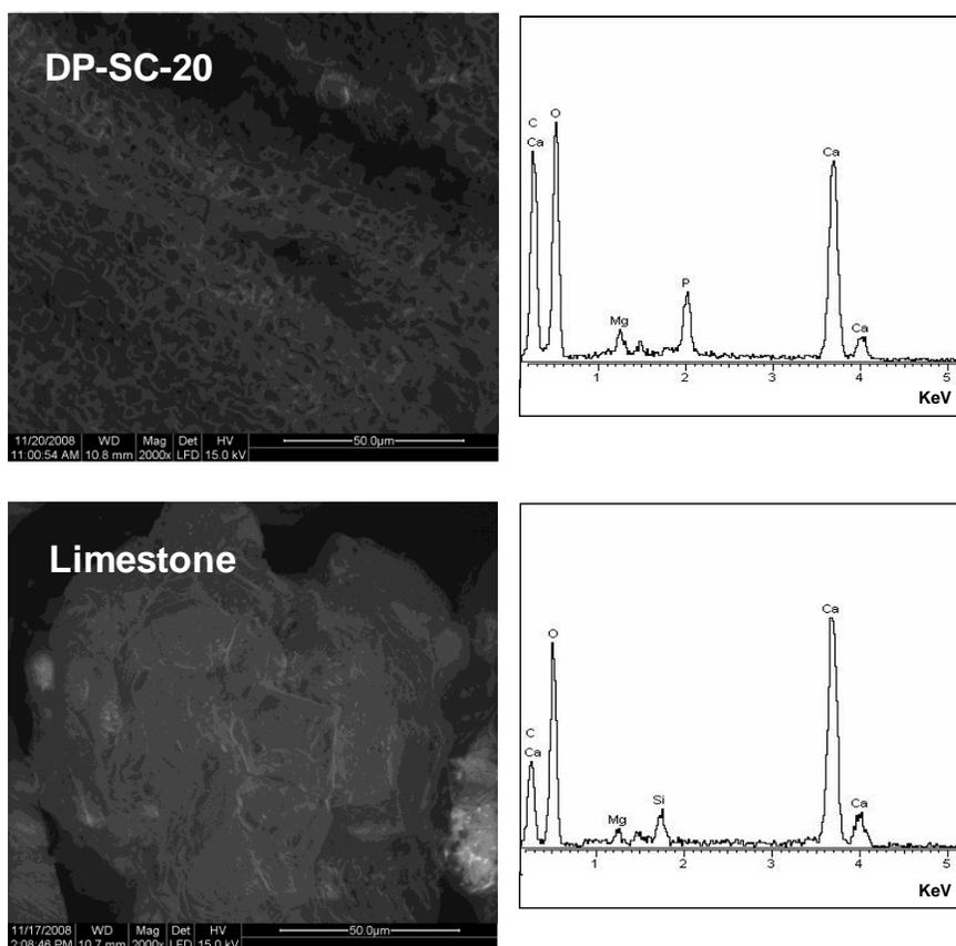
Figure 1. SEM micrographs and EDS spectra of DP-SC20 and limestone.
