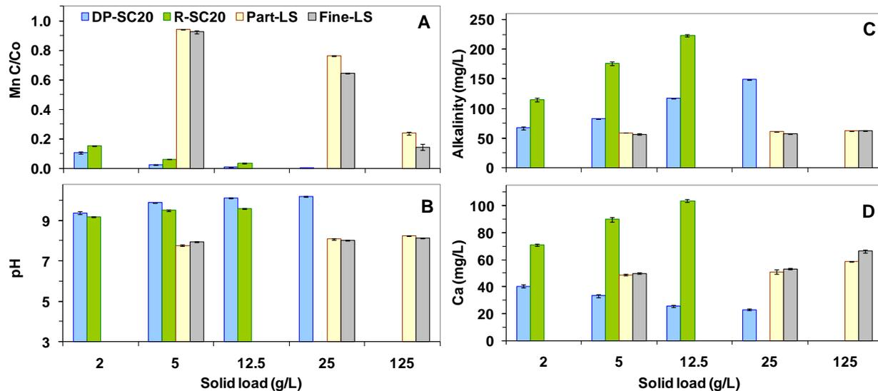
Figure 2. Final manganese concentration (A), pH (B), alkalinity (C), and calcium (D) in systems containing SMIW with initial Mn of 10 mg/L and pH 3.0, treated with DP-SC20, R-SC20, particulate limestone (Part-LS), and fine limestone (Fine-LS). Values represent triplicate averages; error bars represent one standard deviation.
