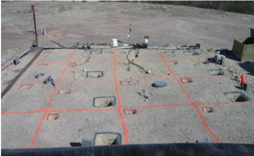
Figure 1. Photo of the top covered surface of the waste rock pile. The large grid (orange) lines approximate the 2×2m boundaries of underlying lysimeters. The smaller (16 red and 8 blue) squares mark the locations of sample pits and density test pits respectively.
