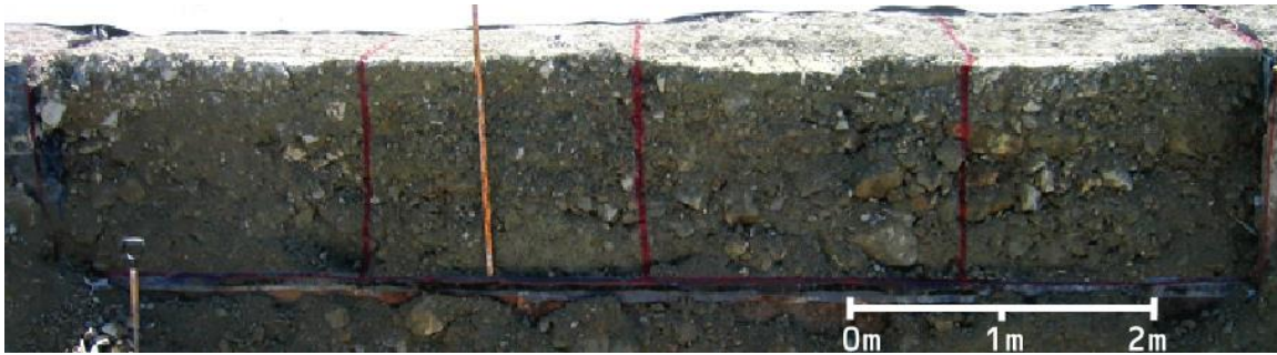
Figure 2. Photo of a vertical trench face at the base of the experimental waste rock pile. Vertical (red) lines approximate boundaries of underlying lysimeters. Note the heterogeneity in waste rock texture.
