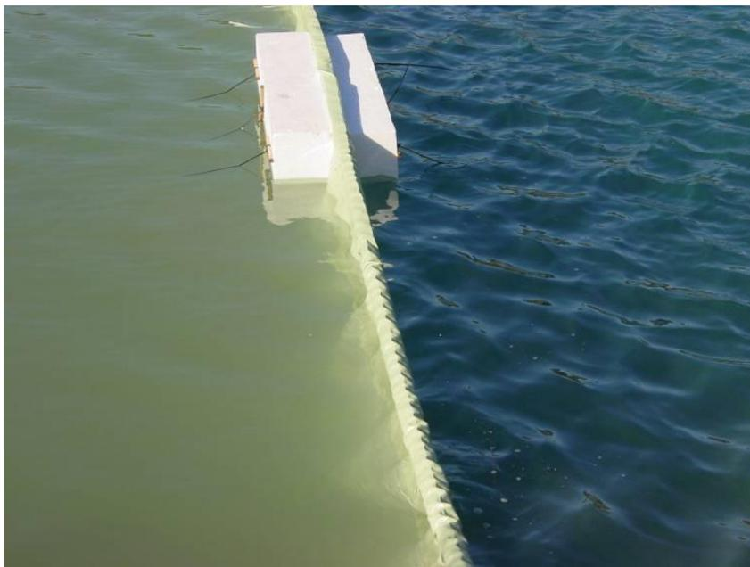
Figure 4. Photograph taken in May 2003 showing the effectiveness of the barriers in isolating the macrocosms
