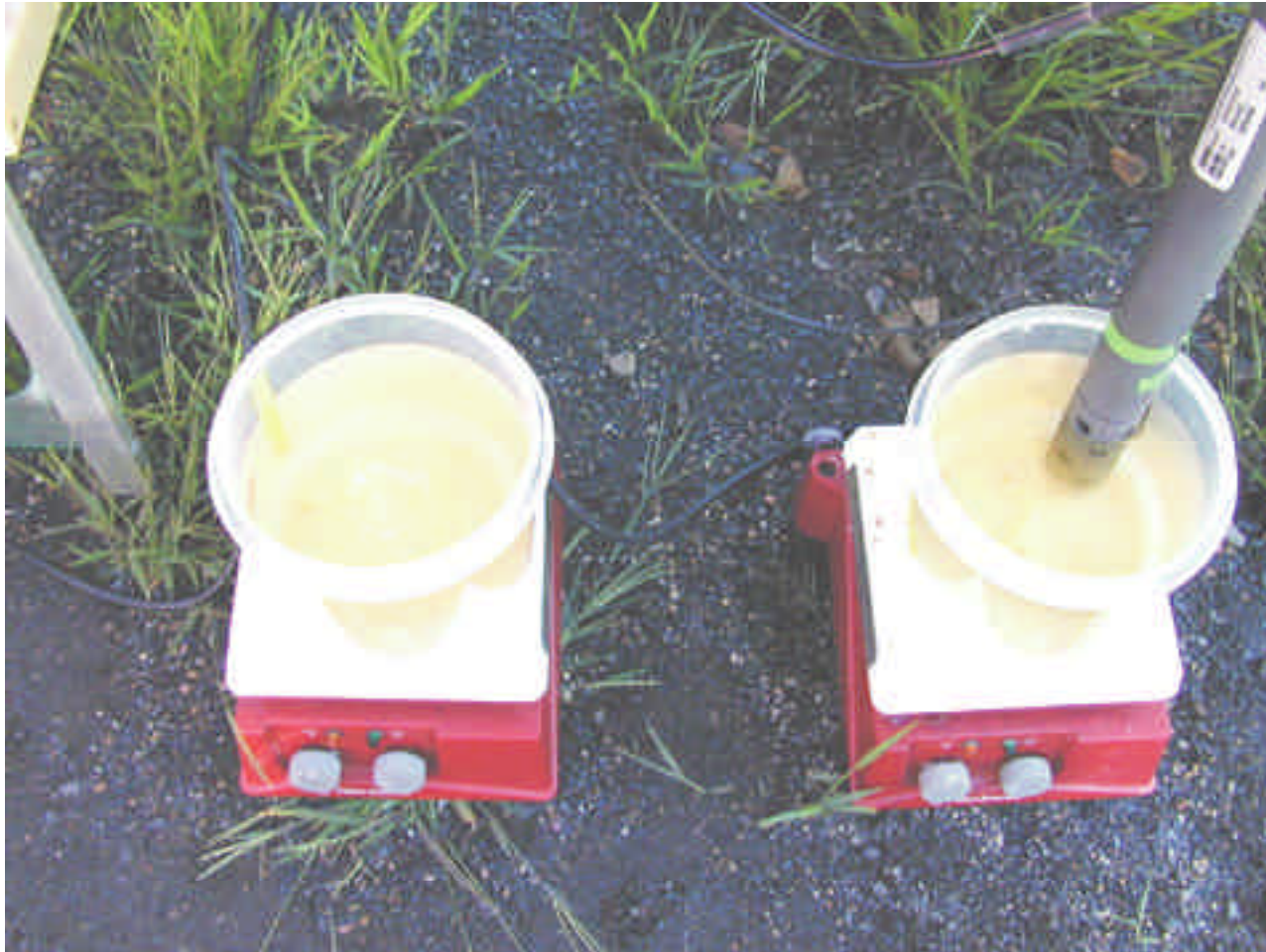
Figure 1. Water ( \pm iron oxides and bacteria) for all experiments was collected in the field. Some oxidation experiments were conducted in the field as shown, and some were conducted in the lab soon after transport. DO, pH, and T were measured with a YSI multimeter (shown). Most experiments were less than one hour duration (with the exception of BR 31-34). No sediments were added to the experiments shown here.
