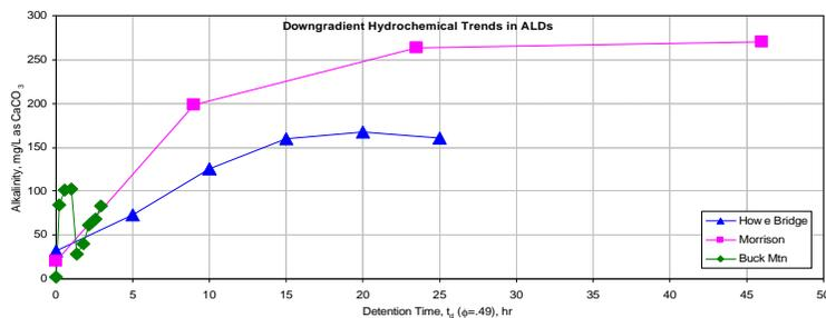
Figure 1. Changes in alkalinity concentration with detention time (downflow distance) of mine drainage within limestone drains at Howe Bridge, Morrison, and Buck Mtn. sites. Detention time computed as product of porosity ( $f$ ), downflow distance ( $L$ ), and cross-sectional area ( $A$ ) divided by flow rate ( $Q$ ):  $t_d = f \cdot L \cdot A / Q$ , assuming  $f = 0.49$ .
