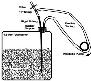
**Figure 4. Schematic of polyethylene "cubitainder" containing 4 kg limestone and filled with mine discharge water to evaluate alkalinity production rates (after Watzlaf and Hedin, 1993).**
