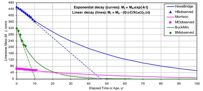
**Figure 2. Decline in mass of limestone with age of limestone drain. Solid curves indicate continuous dissolution on the basis of Eq. (1) and rate constants (k) derived from field data (Table 2, Fig. 3). Dashed lines indicate decay trends for constant alkalinity flux. Measured data points from Table 2.**
