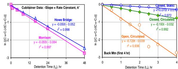
**Figure 6. Natural logarithm of difference between steady-state maximum alkalinity ( $C_M$ ) and measured alkalinity ( $C_t$ ) divided by difference between  $C_M$  and initial alkalinity ( $C_0$ ) versus time for cubitainder tests for Howe Bridge, Morrison, and Buck Mtn. Sites. Negative value of slope indicates rate constant ( $k'$ ) for computation of alkalinity as a function of detention time ( $C_t$ ) on the basis of Eq. (3):  $C_t = C_0 + (C_M - C_0) \exp(-k' \cdot t_d)$ .**
