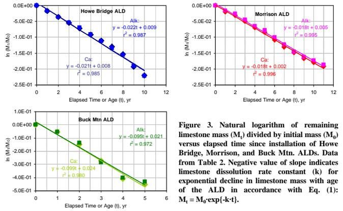
**Figure 3. Natural logarithm of remaining limestone mass ( $M_t$ ) divided by initial mass ( $M_0$ ) versus elapsed time since installation of Howe Bridge, Morrison, and Buck Mtn. ALDs. Data from Table 2. Negative value of slope indicates limestone dissolution rate constant (k) for exponential decline in limestone mass with age of the ALD in accordance with Eq. (1):  $M_t = M_0 \exp(-k \cdot t)$ .**
