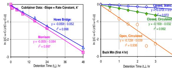
**Figure 6. Natural logarithm of difference between steady-state maximum alkalinity ( $C_M$ ) and measured alkalinity ( $C_t$ ) divided by difference between  $C_M$  and initial alkalinity ( $C_0$ ) versus time for cubitainder tests for Howe Bridge, Morrison, and Buck Mtn. Sites. Negative value of slope indicates rate constant ( $k'$ ) for computation of alkalinity as a function of detention time ( $C_t = C_M - [(C_M - C_0) \exp(-k' \cdot t_d)]$ ).**
