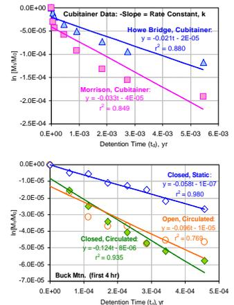
**Figure 7. Natural logarithm of remaining limestone mass ( $M_t$ ) divided by initial mass ( $M_0$ ) versus initial elapsed time of cubitainder tests for Howe Bridge, Morrison, and Buck Mtn. ALDs. Remaining mass computed by subtracting cumulative flux of CaCO<sub>3</sub> from the initial limestone mass and dividing by limestone purity. Negative value of slope indicates first-order rate constant (k) for exponential decline in limestone mass with age of the ALD on the basis of Eq. (1).**
