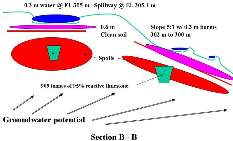
Figure 13. The subsurface aspects of the reclamation-restoration design in Knights Branch.
