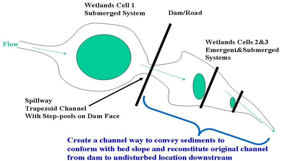
Figure 19. Added design features along Knights Branch to match hydrology to the geomorphic features of the valley.
