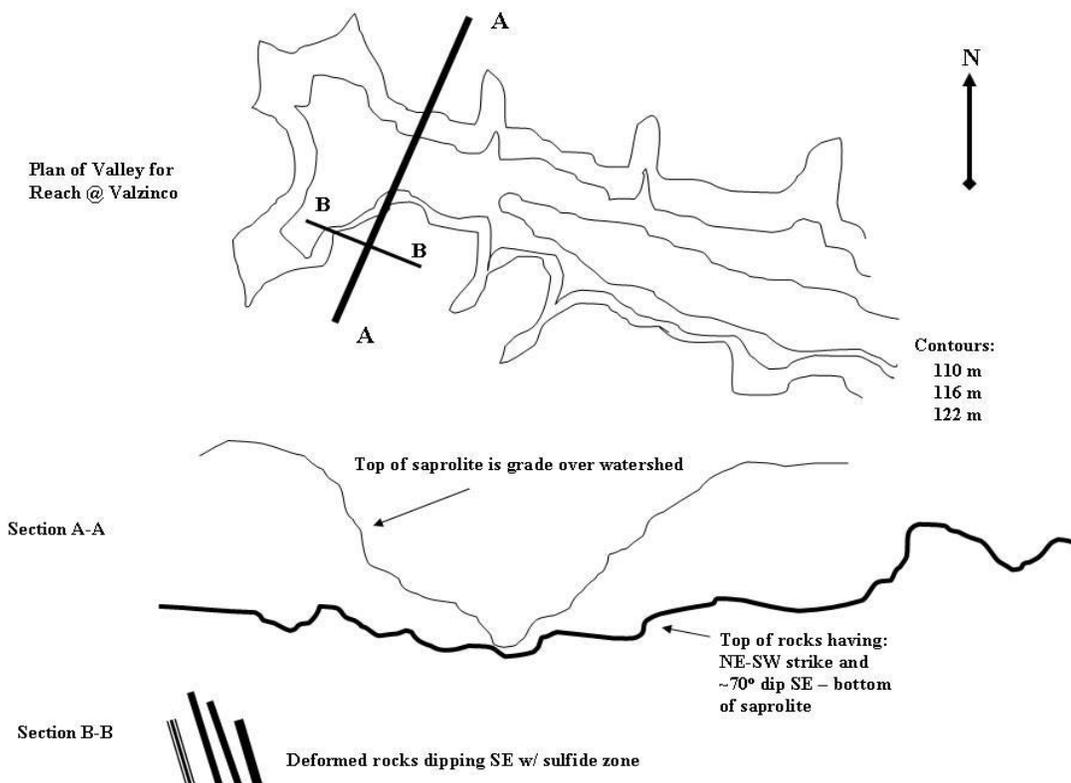
Figure 2. Arrangement of saprolite in Knights Branch at Valzinco Mine.
