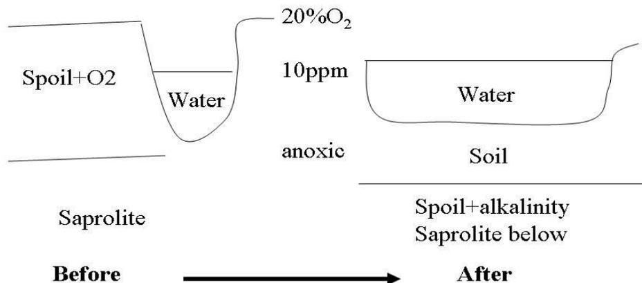
Figure 11. Conceptual design for the conditions in Knights Branch watershed at Valzinco above and below the dam site.
