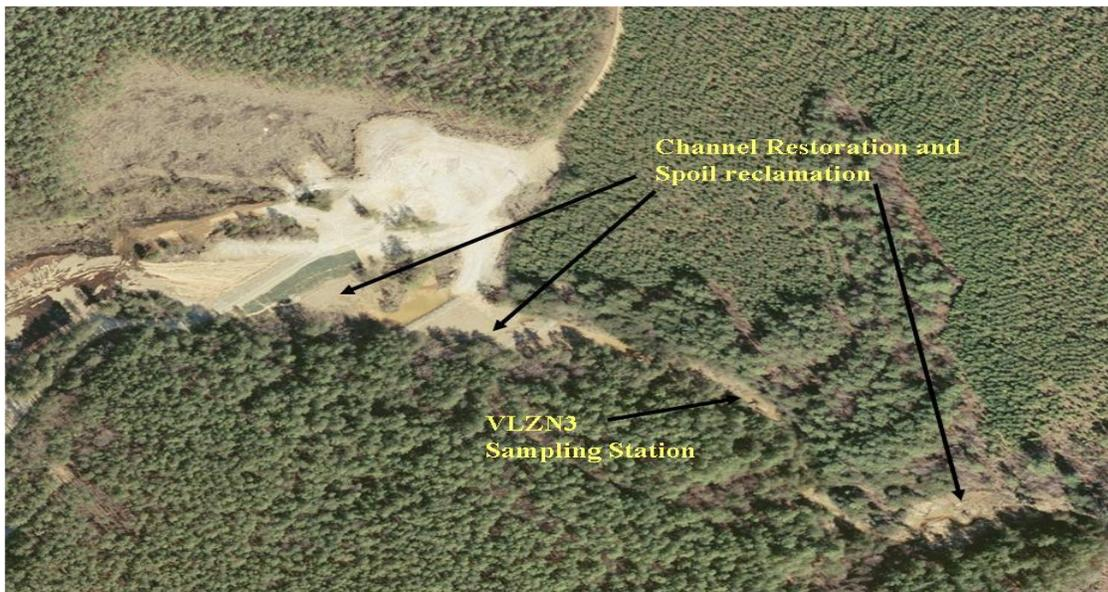
Figure 18. Phase II establishes a southern channel for Knights Branch from the dam through Wetlands Cell 2.
