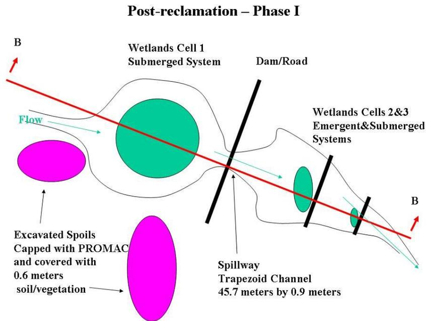
Figure 12. The surface design for reclamation of Valzinco Mine and restoration of Knights Branch.
