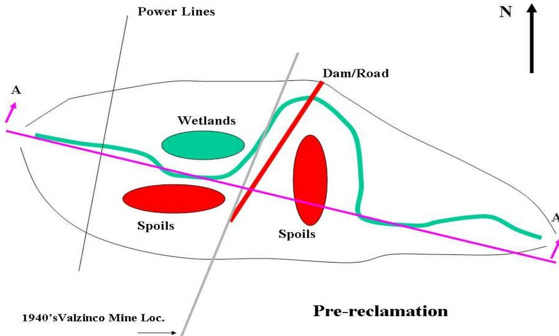
Figure 9. Position of stream channel after mining operations ceased at Valzinco.
