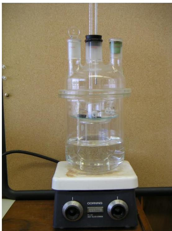
Figure 1. Setup of weathering chamber used in the simulated weathering experiments.
