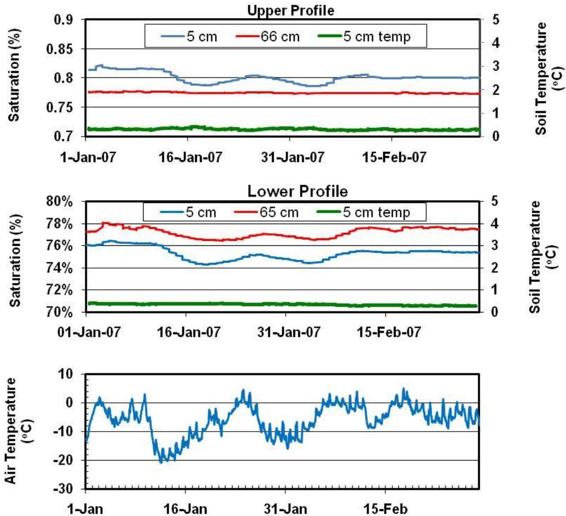
Figure 6. Changes in degree of saturation and soil temperature at two cover profiles in response to air temperature changes.
