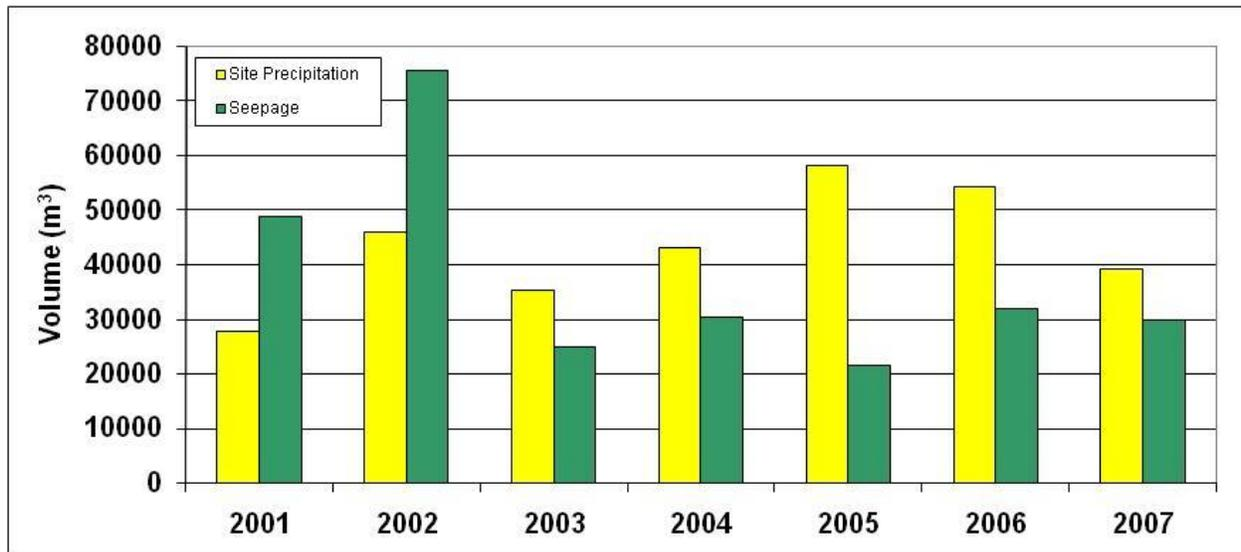
Figure 9. Total annual volume of seepage and precipitation that falls over the dump area. Seepage receives contributions from sources other than direct precipitation; cooling water is likely responsible for seepage volumes exceeding site precipitation in 2001-2002.
