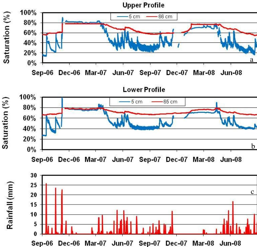
Figure 5. Upper and Lower profile soil cover degree of saturation at a depths of 5 cm and of 65/66cm of the cover (a and b) and rainfall (c).
