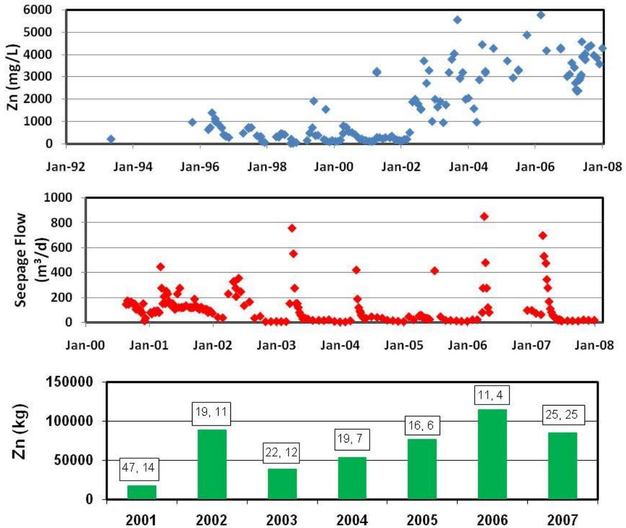
Figure 10. Zinc concentrations (a), Seepage flow rates (b), and Annual zinc mass in seepage (c). The two numbers above the bars in 9c are the number of flow measurements and chemistry analyses, respectively.
