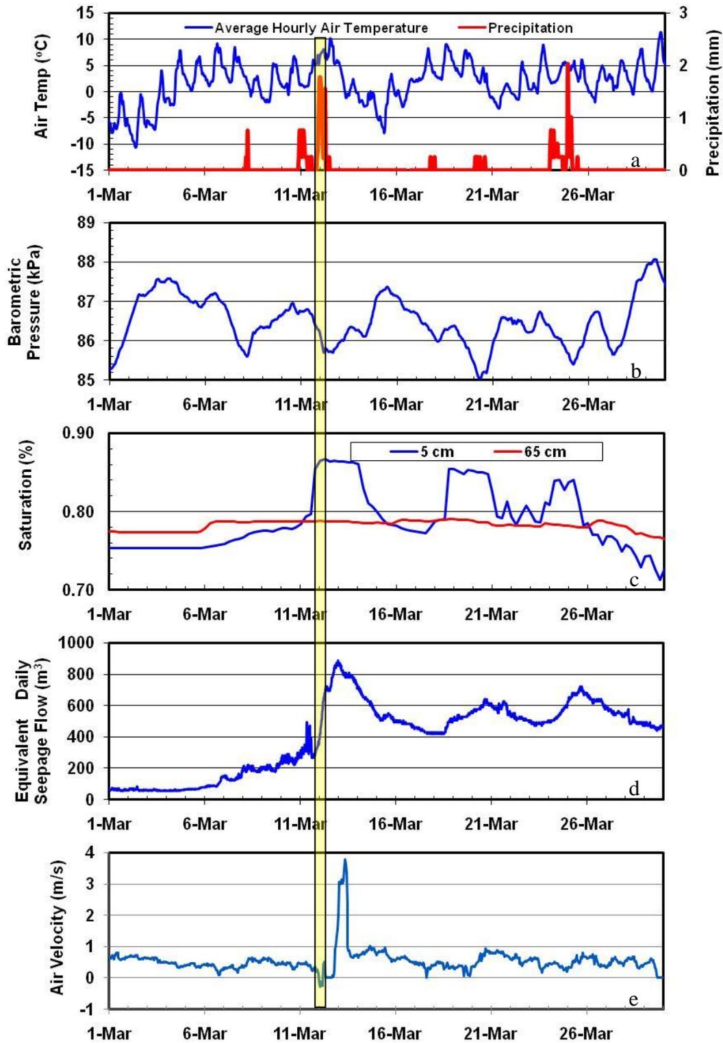
Figure 8. Site parameters from March 2007, highlighted on the period of barometric pressure control of March 12: air temperature and precipitation (a), barometric pressure (b), cover soil saturation (c), seepage flow (d), and air velocity in the 400 mm pipe (e).
