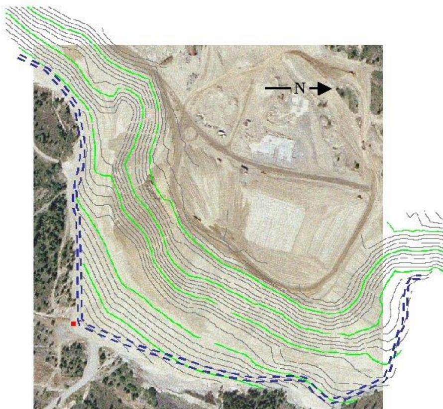
Figure 2. No. 1 Shaft waste dump. The drain, formerly the ditch, is shown with blue dashed lines along the toe. The monitoring station is the red square at the southeast corner of the dump.
