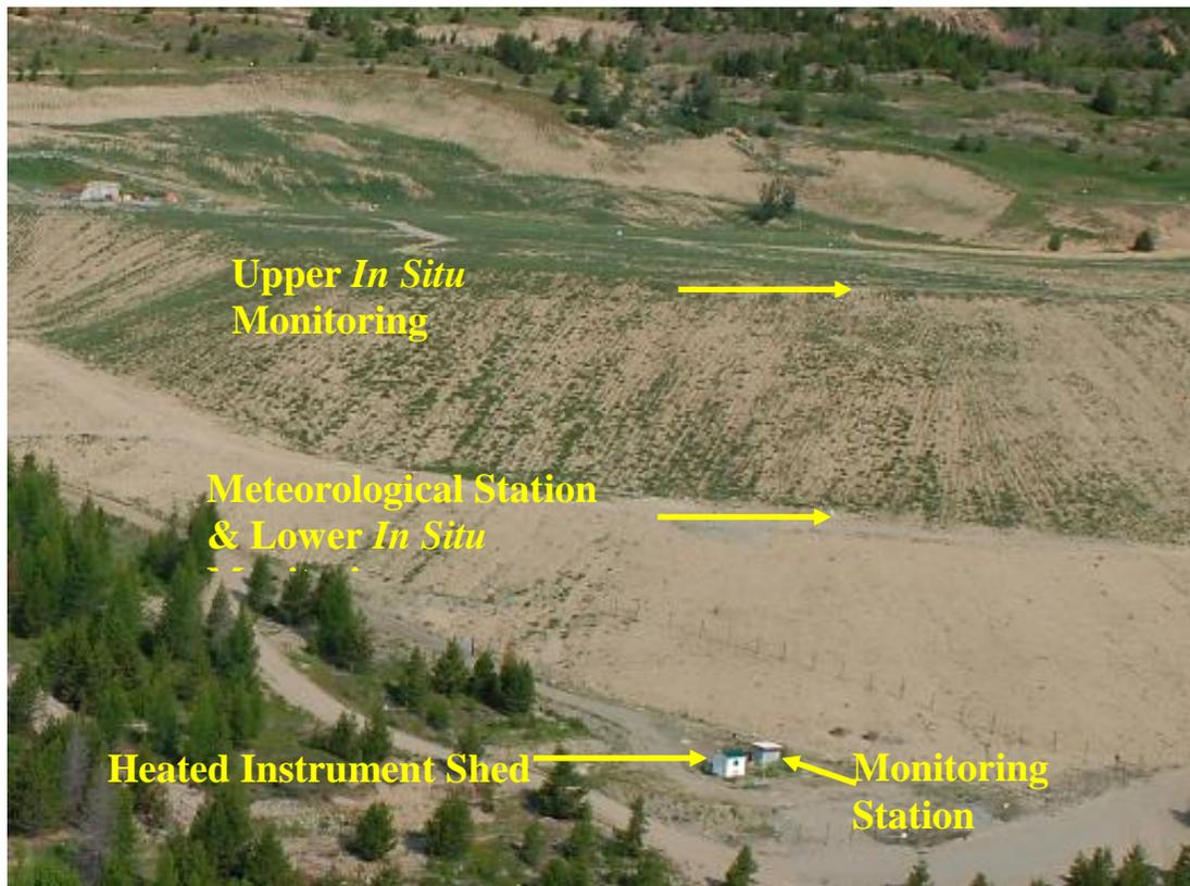
Figure 4. Layout of Phase 1 monitoring system on the No.1 Dump looking northwest (taken July 2008)
