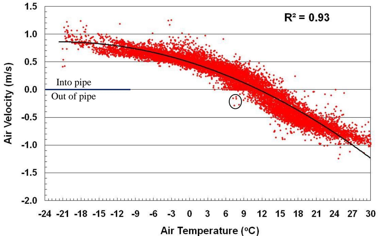
Figure 7. Air Velocity versus Air Temperature in the 400 mm pipe. The data within the oval are from the March 12, 2007 barometric pressure-controlled respiration event.
