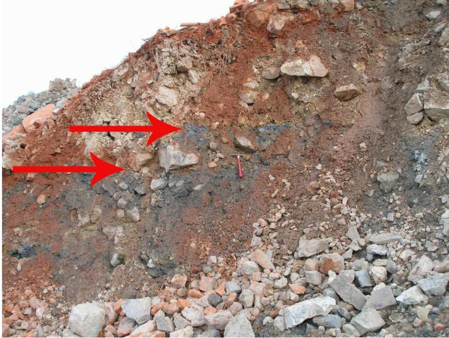
Figure 5. Photo of trench wall cut into the Buttruss after Bauxsol slurry was sprayed onto the surface. Gray layer just above hammer is a lime layer; another is just at the level of the hammer. Red stain is from Bauxsol, but below the lower lime layer it has fallen onto the face from above after the trench was cut. Nearly all Bauxsol is above the lime layers
