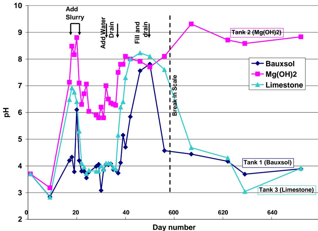
Figure 14. Plot of pH values of effluent from tank experiments, versus day number. Note break in scale at 60 days.
