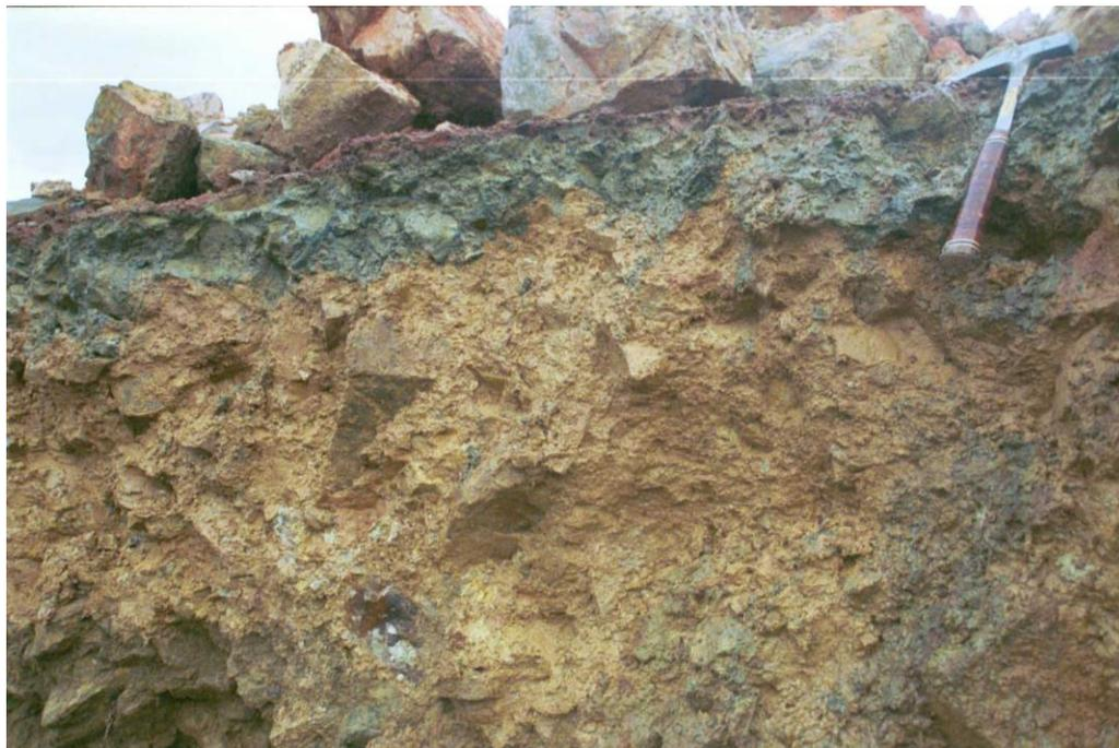
Figure 12. Photo of trench wall excavated in the Buttress area where Bauxsol slurry had been sprayed on the surface. The green zone contains the green rust phase that turned red in a few hours after exposure.
