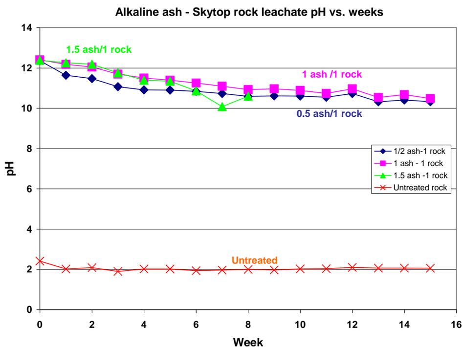
Figure 13. Values of pH in leachates from bucket tests of mixtures of Skytop pyritic rock with alkaline CFB ash, conducted by Meiser and Earlf for Robindale Energy Services, Inc. neighborhood and the traffic that would be generated. As a result, this plan was dropped.
