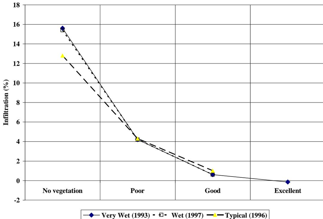
Figure 10. Cumulative infiltration through the cover at the Main monitoring station on the waste rock dump.
