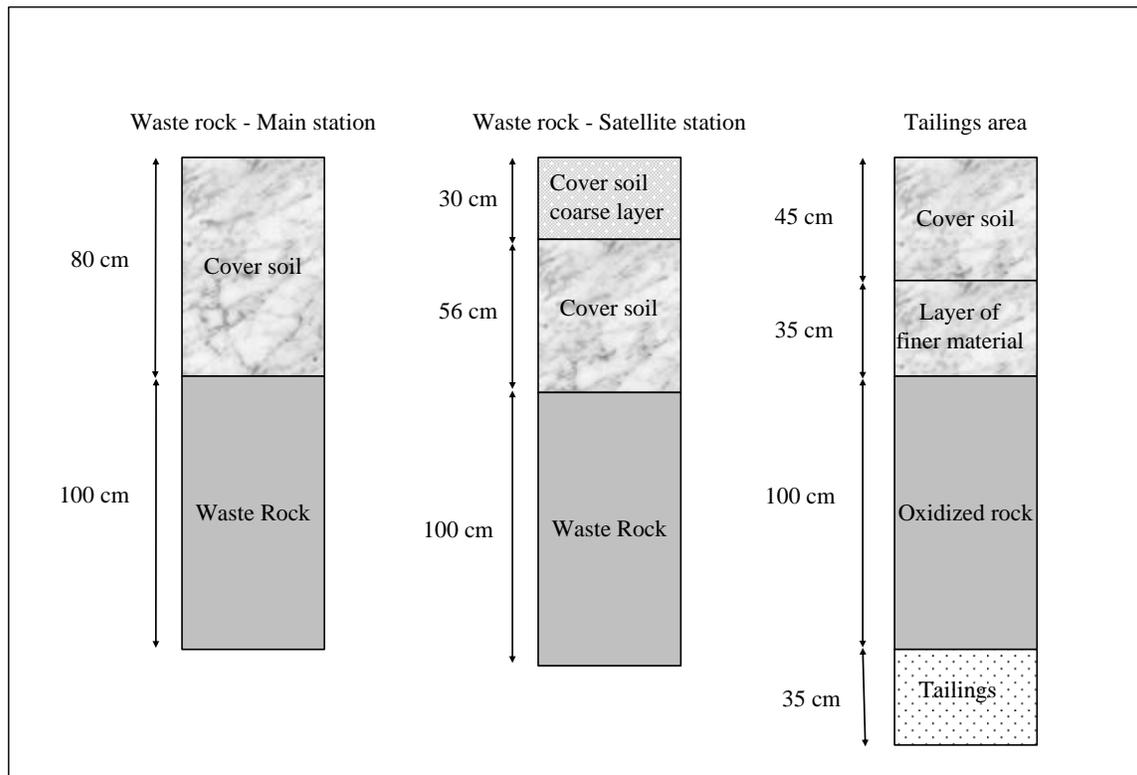
Figure 2. Basic profiles used in the numerical modeling for the waste rock dump and tailings area.
