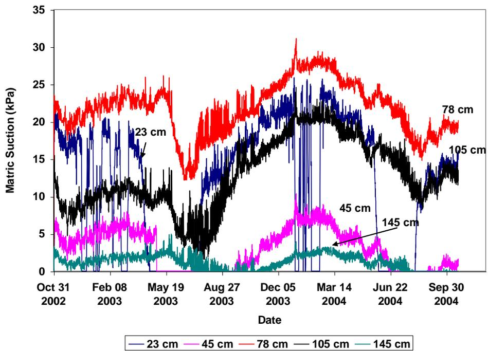
Figure 9. Matric suctions at the tailings monitoring station.
