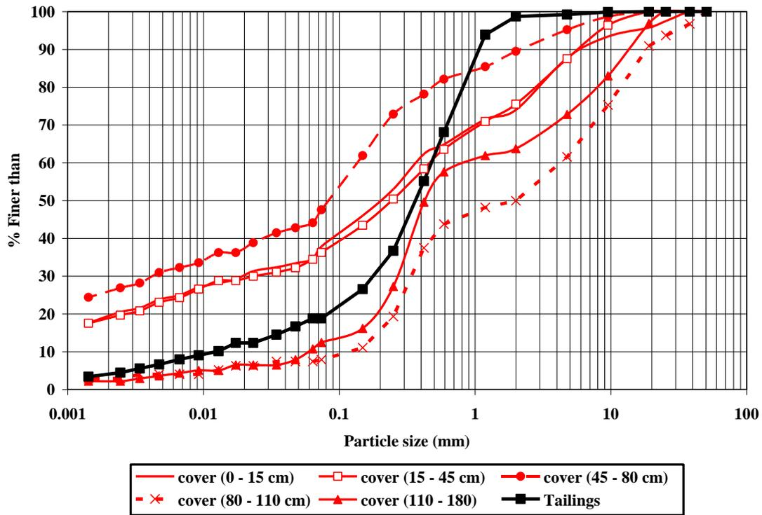
Figure 5. Grain size distribution of the cover system at tailings area.
