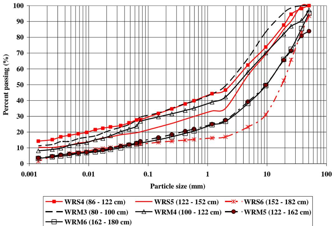
Figure 4. Grain size distribution of waste rock materials
