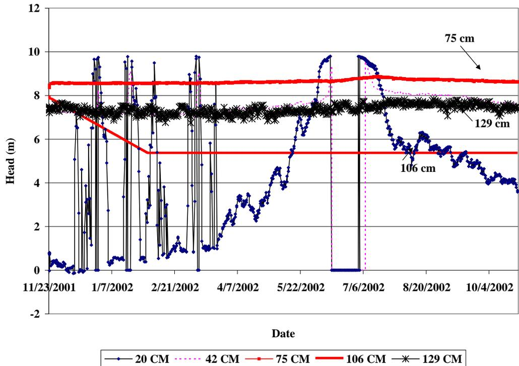
Figure 12. Hydraulic head for the profile at the *Main* monitoring station on the *waste rock dump*.
