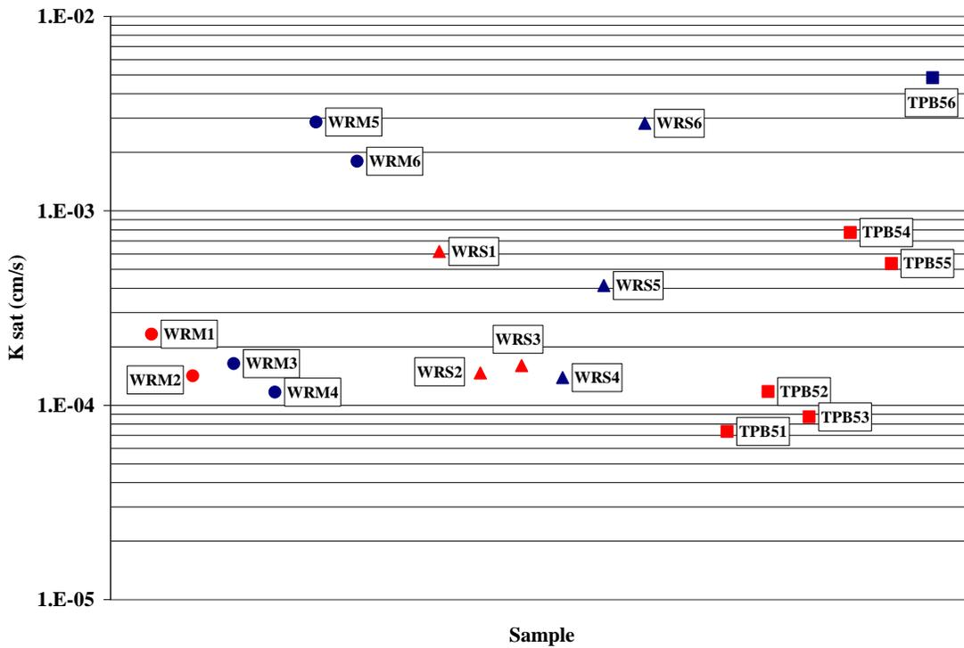
Figure 6. Saturated hydraulic conductivity of the cover systems, waste rock and tailings. Red marks are cover materials and black marks are waste rock and tailings.
