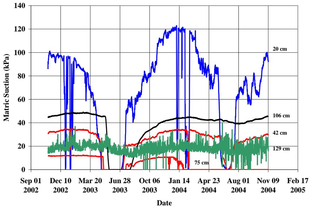
Figure 8. Matric suctions in the cover for the waste rock dump.
