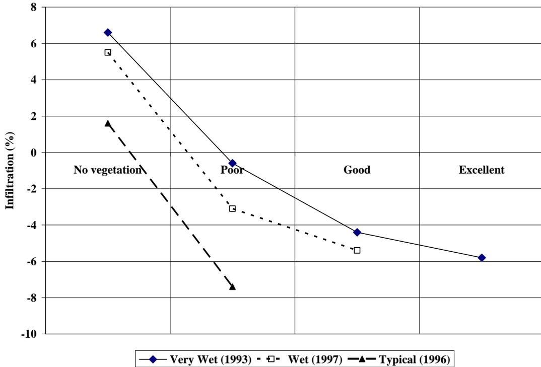
Figure 11. Infiltration rates at the tailings area for different climate and vegetation conditions.
