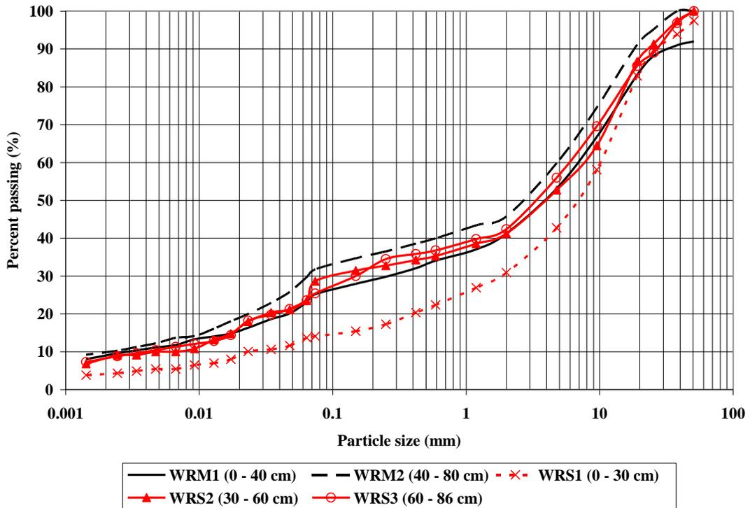
Figure 3. Grain size distribution of the waste rock cover material at the main (WRM) and satellite locations (WRS).
