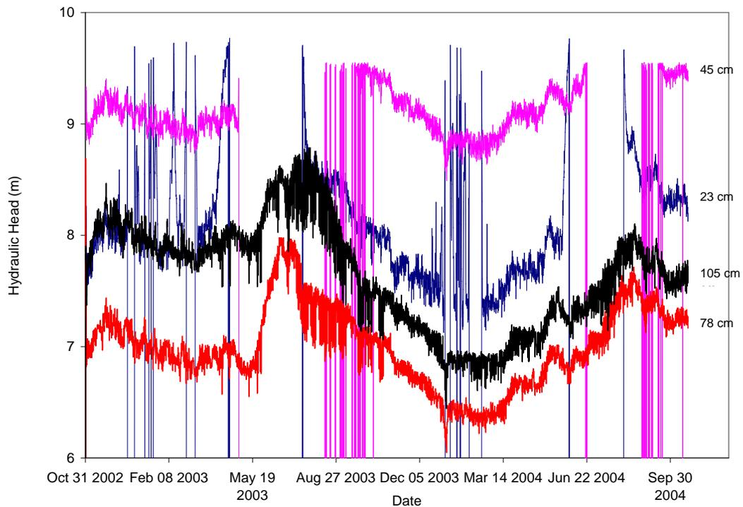
Figure 13. Calculated hydraulic head for the cover system profile at the *tailings* area using actual TC sensors data.
