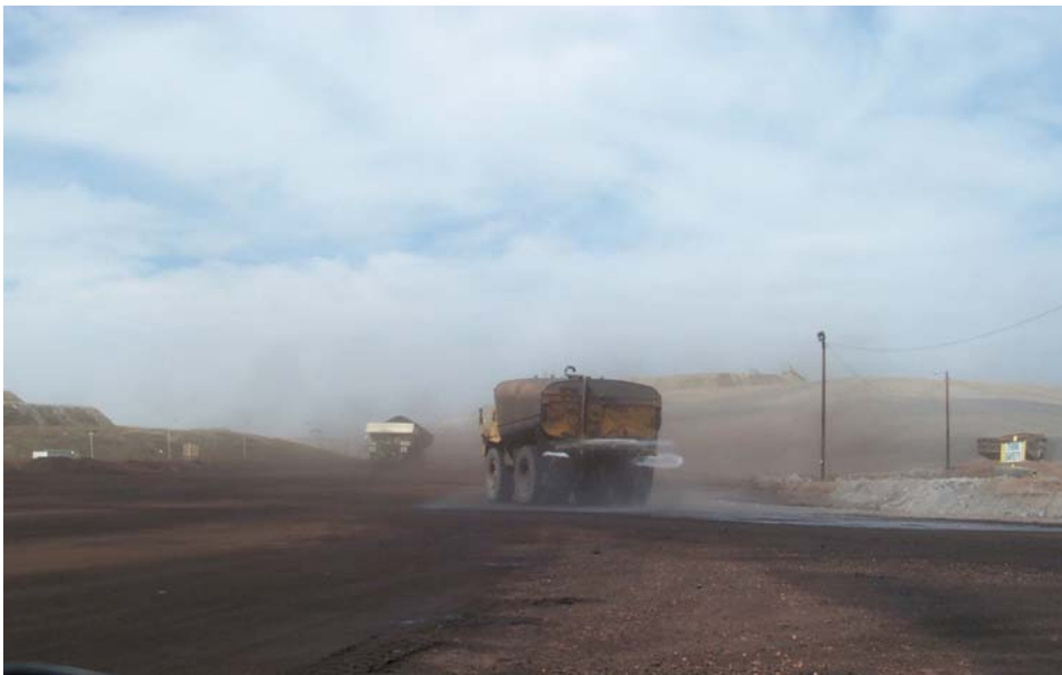
Figure 3: 166 m 3 Water Truck in Operation in Coal Hopper Area During Windy Day.
