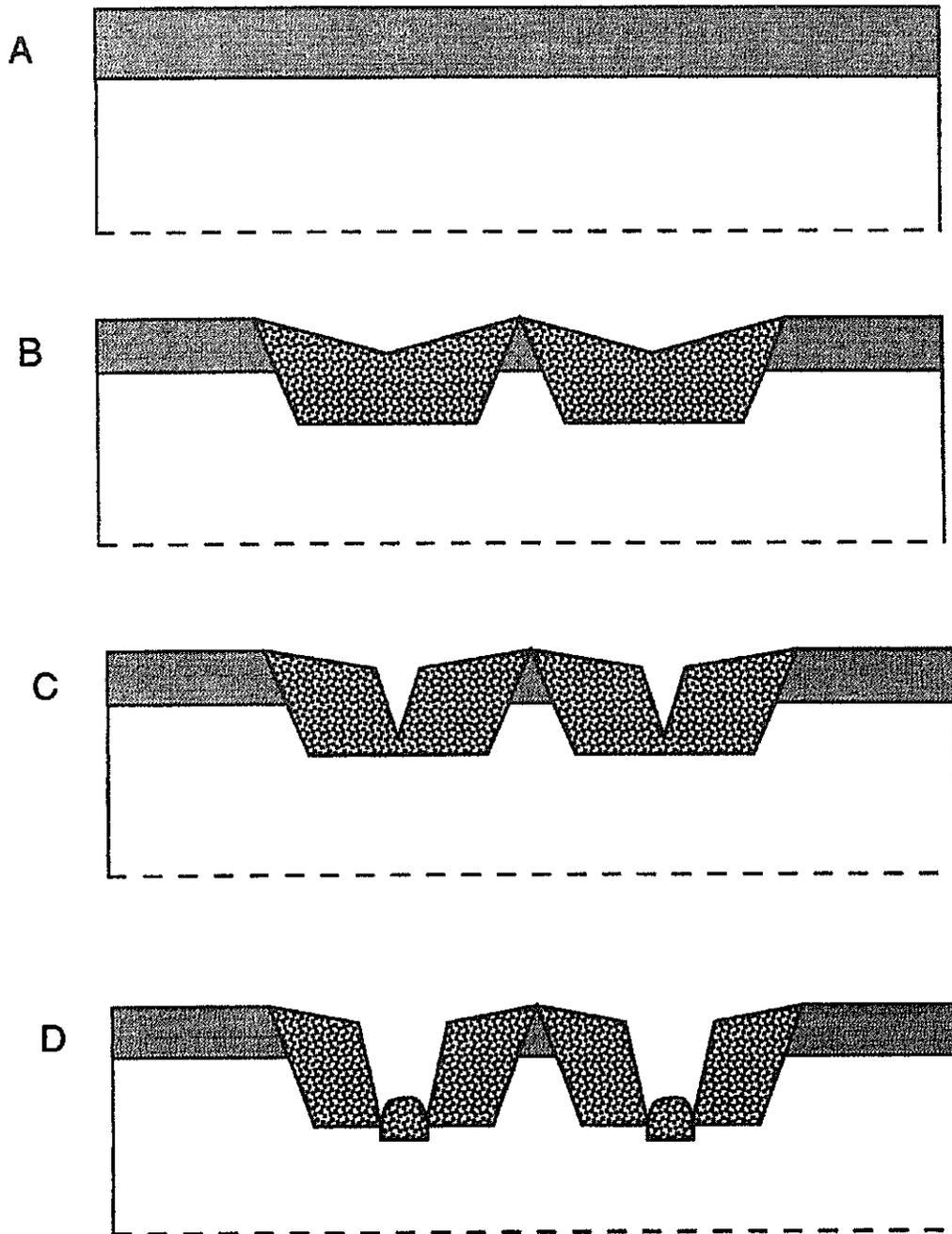
Figure 3: Diagram representing a sequence of hillslope-development processes near Denver, Colorado; (A) horizontal resistant rocks overlying less resistant rocks, forming a mesa-type topography; (B) erosion of sideslopes and filling of gullies with coarse colluvium; (C) fluvial incisement of colluvium; (D) fluvial sorting and additional accumulation of the coarse colluvium, thereby providing the potential for continuing gully-gravure processes.
