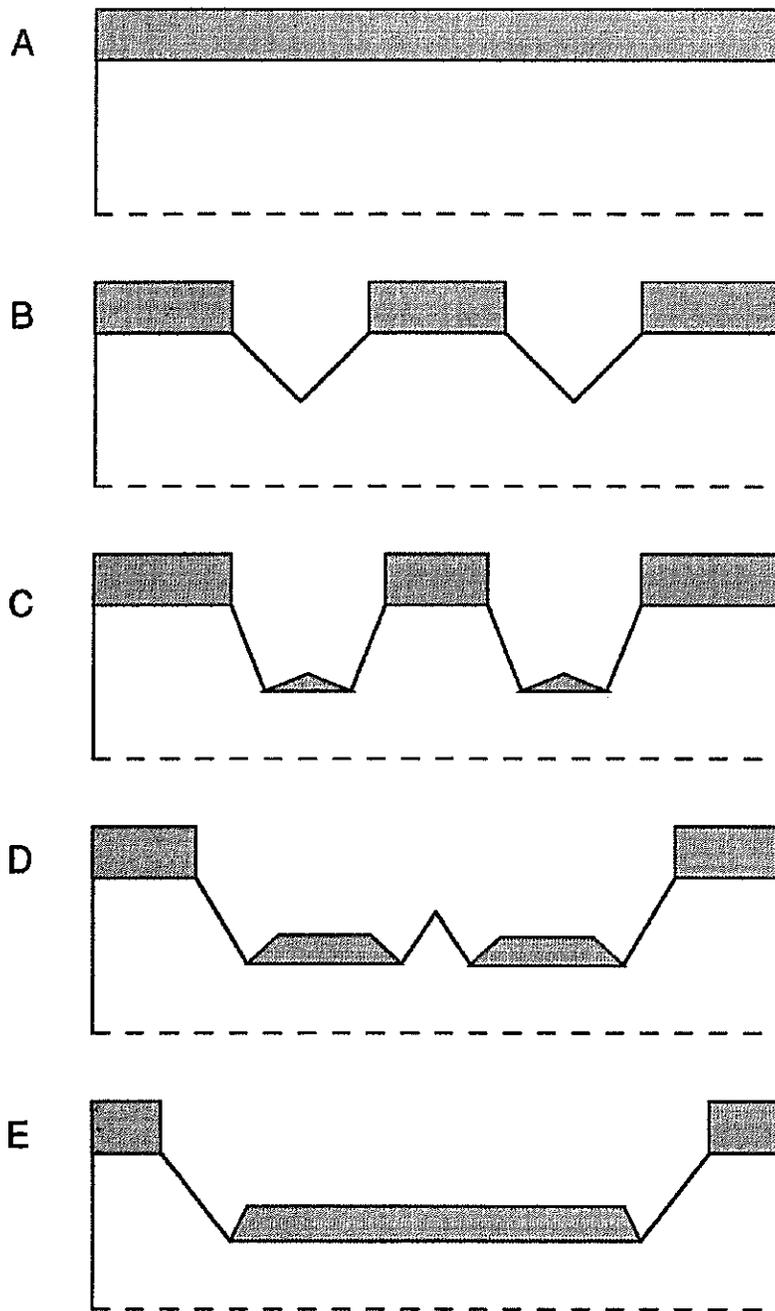
Figure 1: The sequence of gully gravure processes; (A) initial stage of coarse material overlying finer material; (B) incisement of surface by rills and gullys; (C) accumulation of coarse material from above in the incisement; (D) lateral shifting of rills and gullys and continued accumulation of coarse material; (E) lateral planation and formation of a new surface veneered by coarse material.
