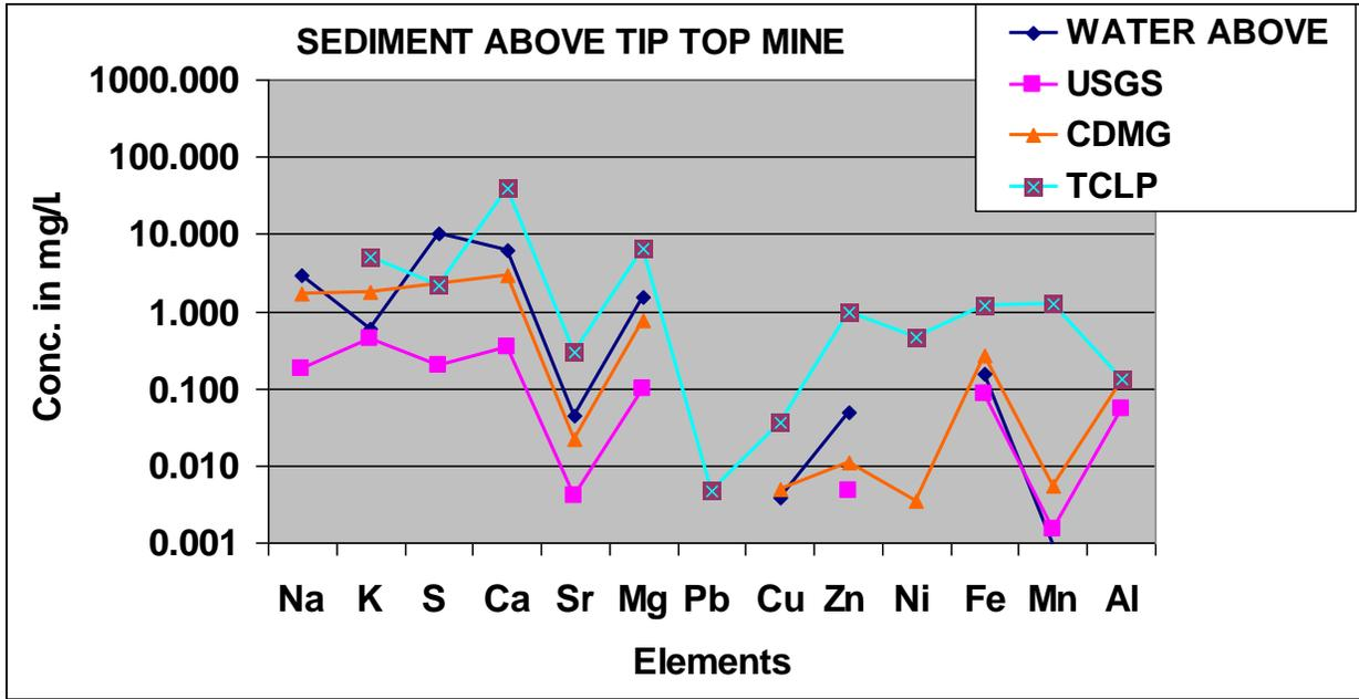
Figure 5. Element Concentration Pattern Graph for the solutions from the three leachate tests for the sediment in Gamble Gulch above the inflow of the Tip Top adit water.
