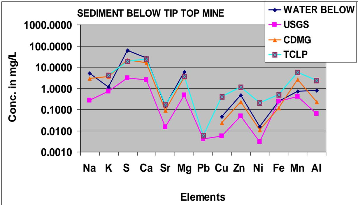
Figure 6. Element Concentration Pattern Graph for the solutions from the three leachate tests for the sediment in Gamble Gulch below the inflow of the Tip Top adit water.
