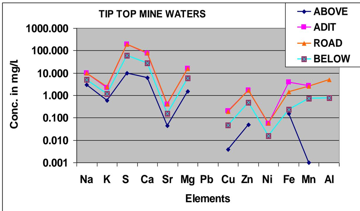
Figure 4. Element Concentration Pattern Graph for the stream waters, the adit water, and the water from the adit at the road 100 meters from the adit at the Tip Top site.
