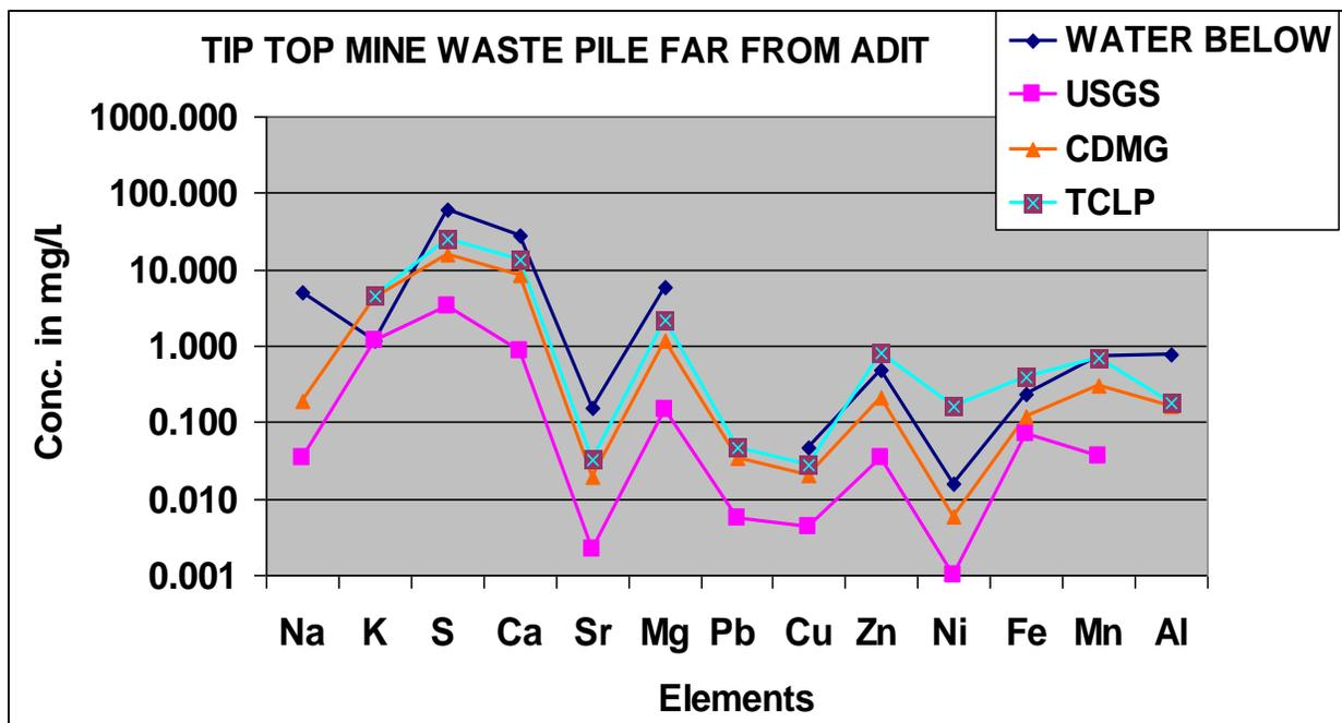
Figure 7. Element Concentration Pattern Graph for the solutions from the three leachate tests for the far waste rock pile at the Tip Top site.
