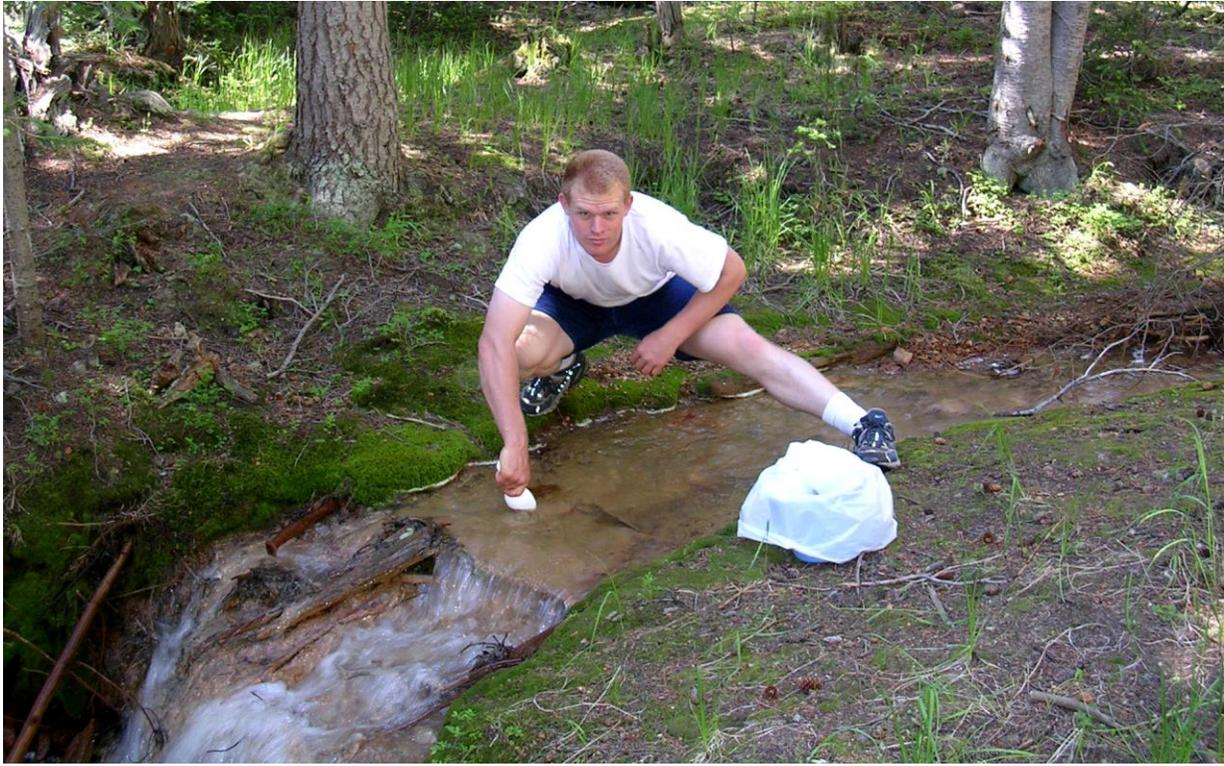
Figure 3. Gamble Gulch below the inflow from the Tip Top adit. Note that the streambed is completely covered with aluminum and iron oxyhydroxide precipitates.
